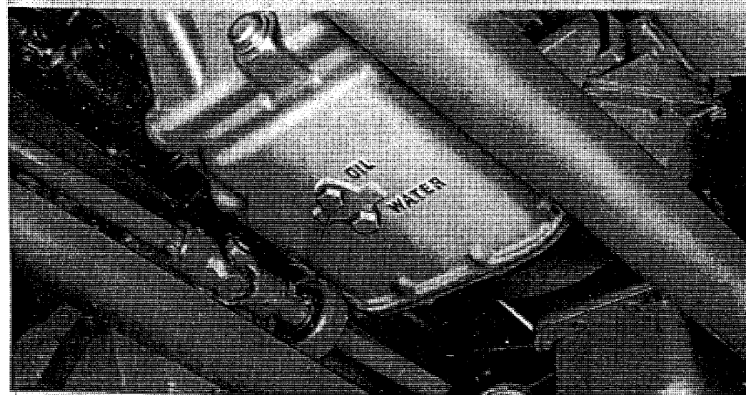
WATER DRAIN PLUG AT TRANSMISSION
