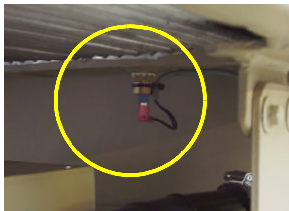
Fig. B.1: Radiator thermo-switch
