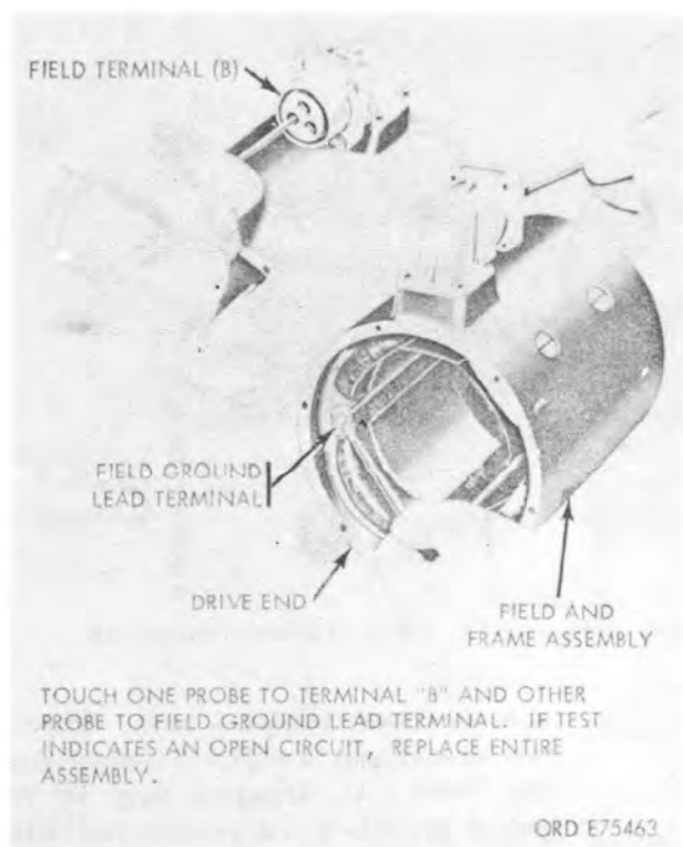
Figure 4-9. Checking housing and windings for open circuits.
