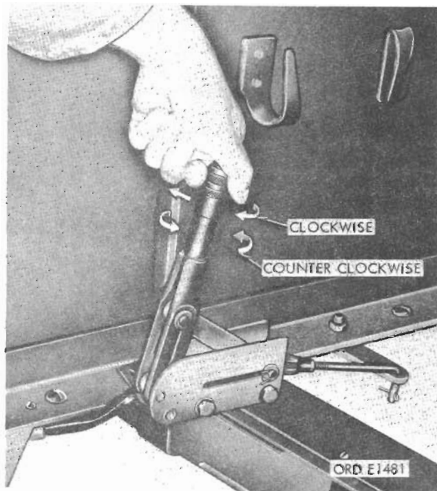
Figure 2-1. Handbrake cable tension adjustment.
