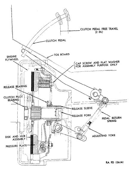
Figure 196. Diagram of clutch and control linkage.
