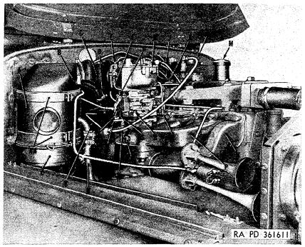
A-Air cleaner body B—Air cleaner outlet hose C-Air-cleaner-to-carburetor inlet hoseD—Hose clamp
