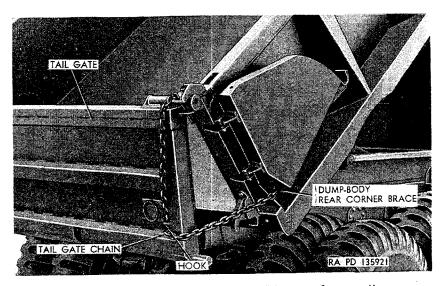
Figure 97. Dump body tailgate arranged for spreader operation.
