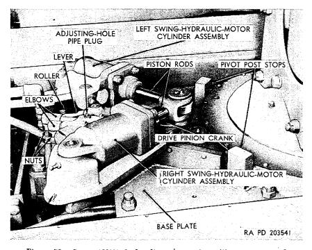
Figure 79. Crane (M62) hydraulic swing motor with cover removed.
