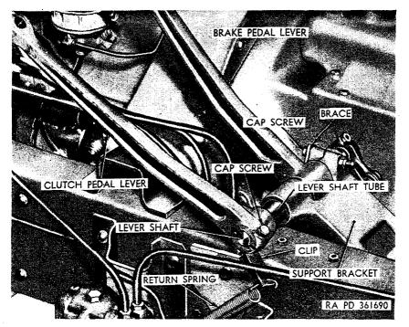
Figure 244. Brake and clutch pedal mounting.
