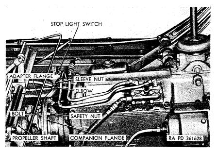
Figure 141. View of right rear section of transmission and transmission-totransfer propeller shaft.
