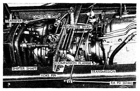
Figure 204. Transmission-to-transfer propeller shaft and shift linkage.
