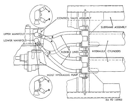
Figure 330. Hoist assembly flexible lines.
