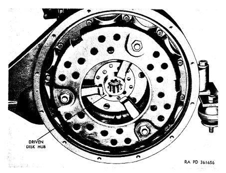
Figure 195. Clutch assembled to engine flywheel.
