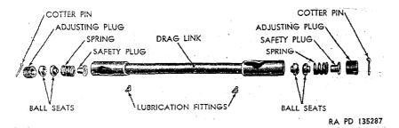
Figure 268. Drag link assembly-exploded view.
