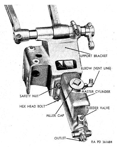
Figure 236. Rear view of brake pedal linkage and master cylinder.
