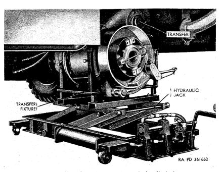
Figure 206. Lowering transfer on hydraulic jack.
