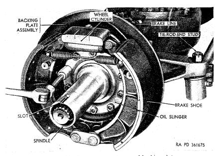
Figure 220. Removing oil slinger and backing plate.
