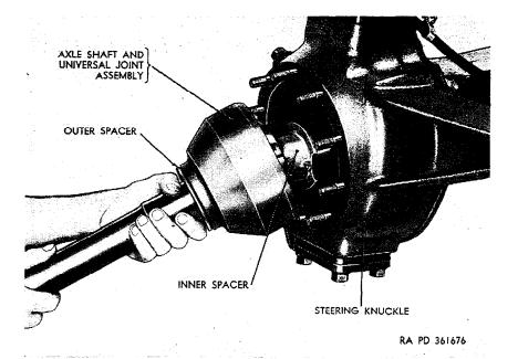
Figure 221. Removing axle shaft and universal joint assembly.
