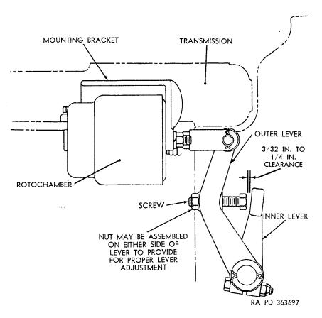
Figure 294. Roto chamber adjustment diagram.
