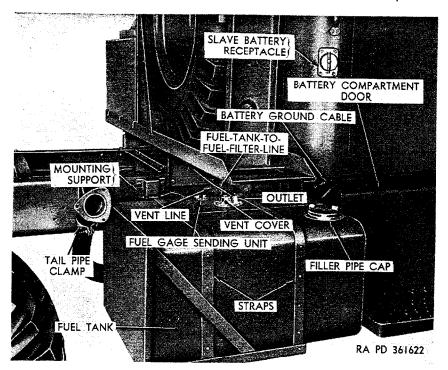
Figure 133.-View of lower right rear corner of truck cub.
