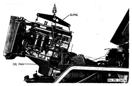
Figure 150. Lifting power plant from truck.
