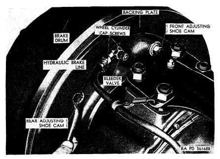
Figure 240. Turning adjusting shoe cam.
