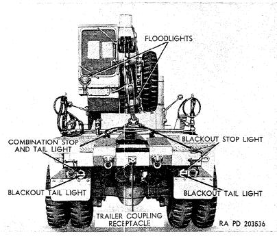
Figure 70. Lights mounted on rear of truck.
