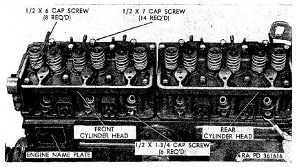
Figure 125. View of left side of engine showing location of head bolts.
