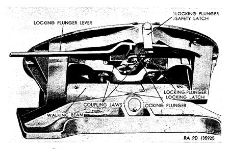
Figure 98. Fifth wheel assembly removed from vehicle-front view.
