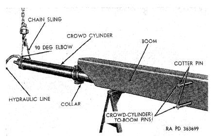
Figure 306. Removing boom crowd cylinder from boom M62 and M246.
