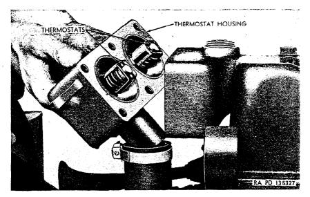
Figure 166. Removing thermostat housing from water outlet header.
