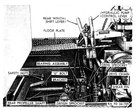
Figure 276. Left side view of rear end of wrecker body with floor plate ruised M26.
