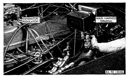
Figure 173. Installing timing adapter at generator regulator.
