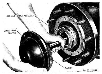
Figure 229. Removing rear axle shaft.
