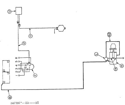
Figure 171. Starting and ignition circuit diagram.
