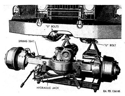
Figure 227. Removing front axle assembly.
