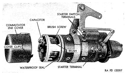
Figure 194. Starter with cover removed.
