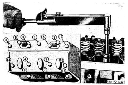
Figure 126. Cytinder head bolt tightening sequence.
