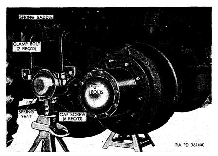
Figure 230. Rear suspension assembly raised for axle removal.
