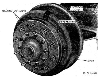
Figure 241. Hub and drum assembly with wheel and tire assembly removed.
