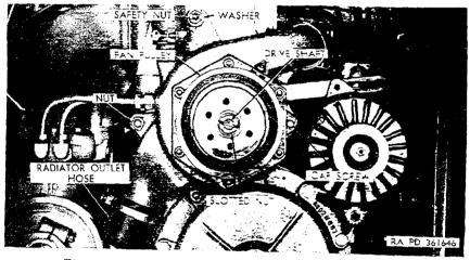
Figure 163. Front view of water pump with fan removed.
