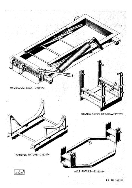
Figure 99. Hydraulic jack and fixtures.
