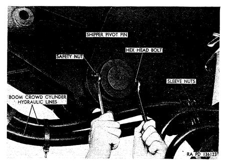
Figure 290. View of right end of shipper pivot pin installed in shipper support.
