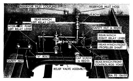
Figure 275. Rear view of forward end of wrecker body with crane removed M62.
