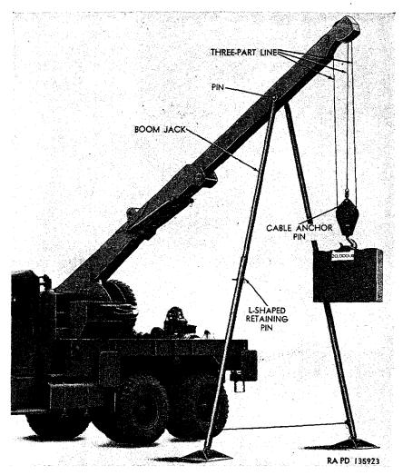
Figure 82. Boom jacks installed (M62).
