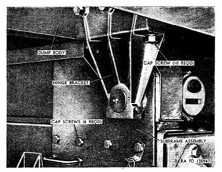
Figure 326. Left rear corner of dump body M51.
