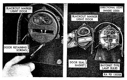
Figure 185. Removing parking lamp and blackout marker lamp.
