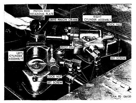
Figure 301. Removing piston rod retaining plate from drive pinion crank M62.
