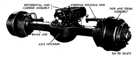
Figure 217. Front axle assembly.
