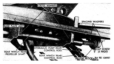
Figure 278. Right side view of underside of crane base plate removed from vehicle M62.
