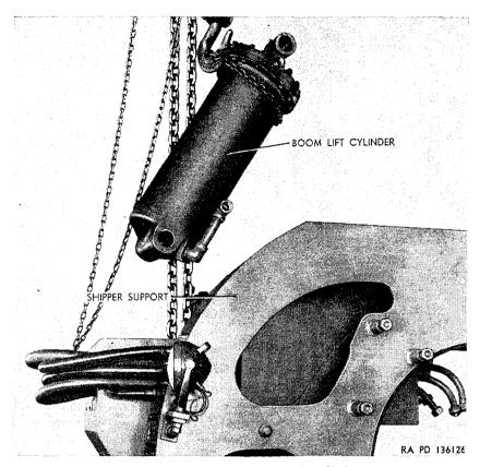
Figure 304. Removing boom lift cylinder.
