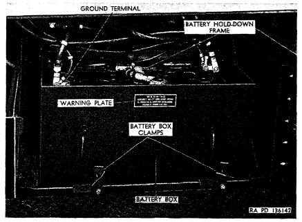
Figure 181. Battery installation.
