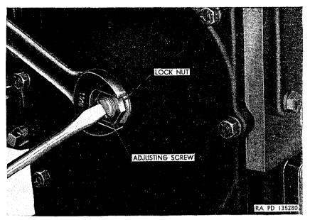
Figure 265. Adjusting pitman-arm shaft.
