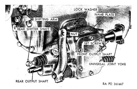
Figure 211. Transmission mounted power-take-off (dump truck M51 only).
