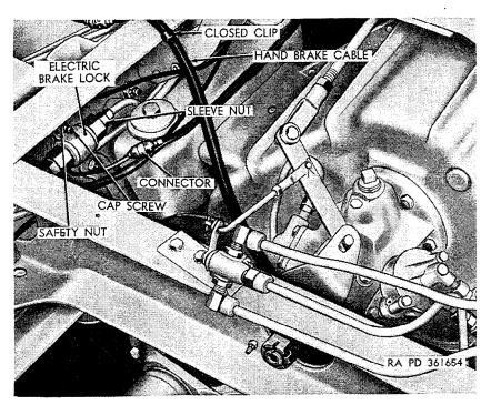
Figure 192. Electric brake lock mounted on frame left side rail.
