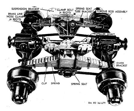
Figure 228. Rear suspension system.
