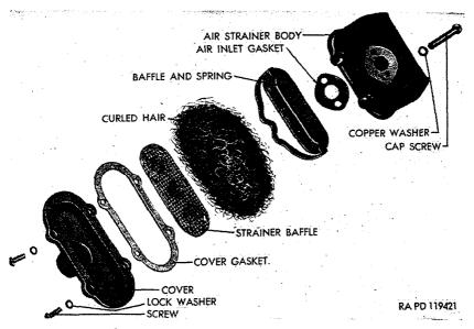
Figure 251. Air-compressor air strainer-exploded view.
