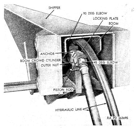
Figure 291. Rear view of boom and shipper assembly with cable drum removed M62.
