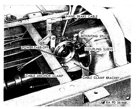
Figure 212. Power-take-off removed from transfer-M62.
