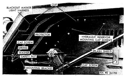
Figure 262. View of underside of left front fender.
