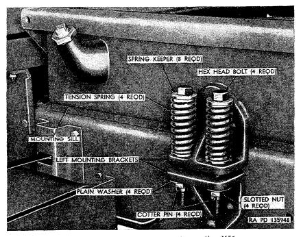
Figure 331. Subframe left front mounting M51.
