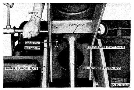
Figure 303. Removing lift cylinder pivot shaft M62.
