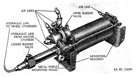
Figure 238. Air-hydraulic cylinder.
