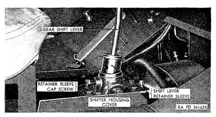
Figure 149. Removing gearshift lever.
