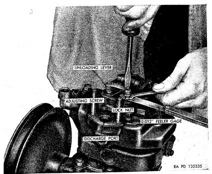
Figure 249. Checking and adjusting air-compressor unloader valve clearances.
