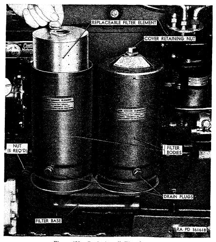
Figure 129. Replacing oil filter elements.
