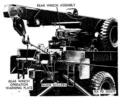
Figure 74. Right rear view of rear winch mounted on vehicle.
