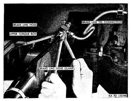
Figure 231. Disconnecting hydraulic brake line hose.
