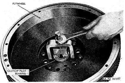
Figure 198. Removing clutch pilot bearing.
