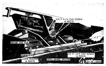
Figure 319. Left front view of fifth wheel M52.
