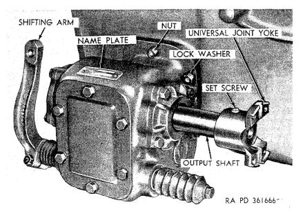
Figure 210. Transmission mounted power-take-off (all models except M51).
