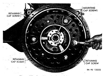
Figure 197. Installing clutch retaining cap screws.
