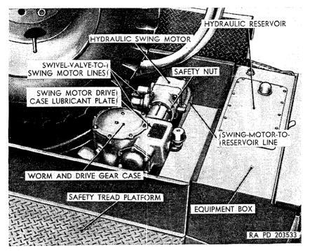
Figure 85. Crane hydraulic swing motor (M246).
