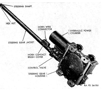
Figure 260. Right side view of steering gear removed from vehicle.
