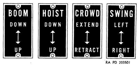
Figure 49. Hydraulic crane control lever instruction plates—models M62 and M246.
