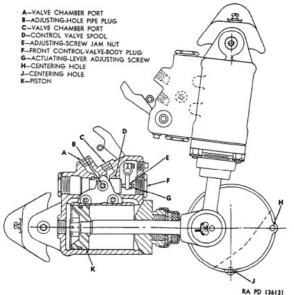
Figure 300. Swing motor timing diagram M62.
