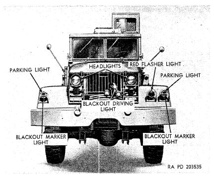
Figure 69. Lights mounted on front of truck.
