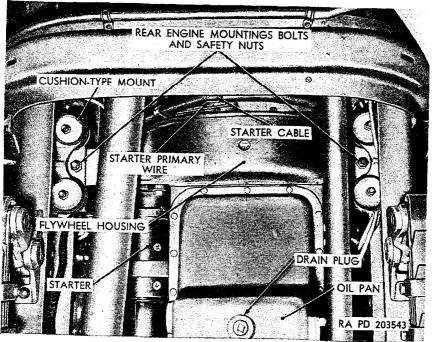
Figure 118. View of rear section of engine from under side of vehicle.
