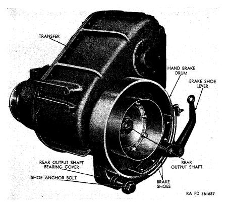
Figure 239. Hand brake mounted on rear of transfer.
