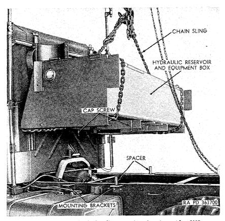
Figure 309. Removing hydraulic reservoir and equipment box M62.
