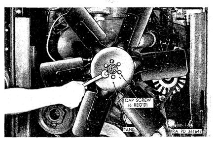
Figure 165. Front view of fan installed on fan pulley.
