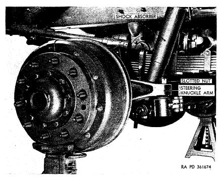
Figure 219. Left end of front axlc assembly with wheel and tire removed.
