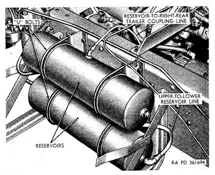
Figure 253. Air reservoirs installed on outside of frame left side rail.
