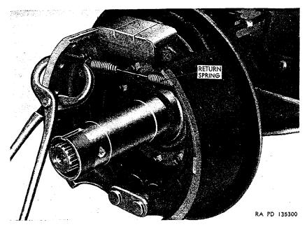
Figure 245. Removing brake shoe return spring.
