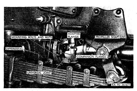
Figure 223. Disconnecting transfer-to-front-axle propeller shaft.
