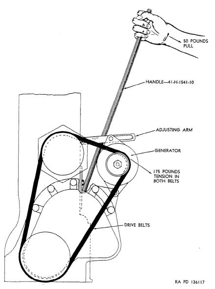
Figure 169. Adjusting drive belts.
