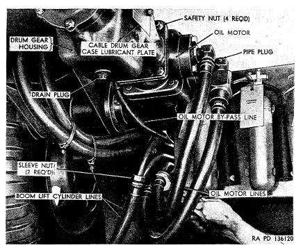
Figure 297. Disconnecting boom hoist hydraulic oil motor lines M62.
