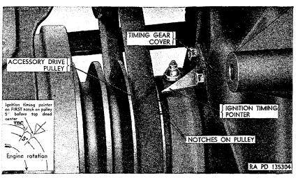
Figure 128. Ignition timing indicator.
