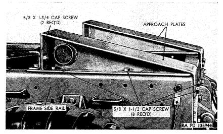
Figure 320. Left rear view of approach plate assembly M52.
