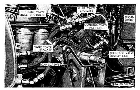
Figure 263. View of steering year installed with left front fender removed.
