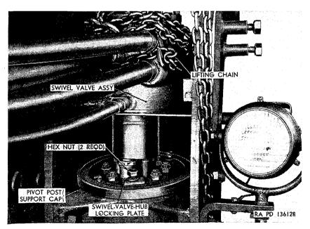
Figure 289. Front view of upper end of pivot post with swivel valve in raised position.
