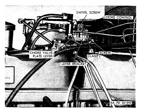
Figure 158. Top left rear view of carburetor installed on engine.
