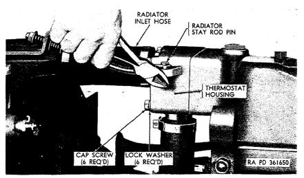
Figure 170. Removing radiator stay rod from thermostat housing.
