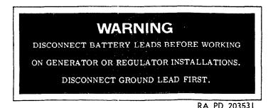
Figure 29. Battery disconnect warning plate.
