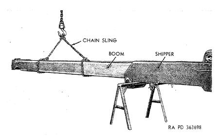
Figure 305. Removing boom from shipper M62.
