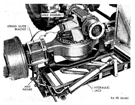
Figure 235. Removing forward rear axle assembly.
