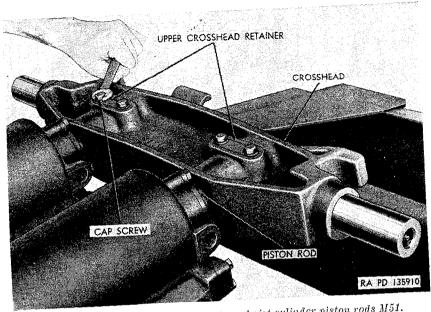
Figure 327. Removing crosshead from hoist cylinder piston rods M51.
