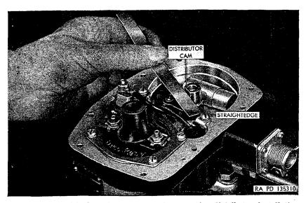
Figure 179. Positioning distributor breaker cam for distributor installation.
