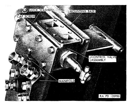
Figure 332. Removing control valve assembly M51.
