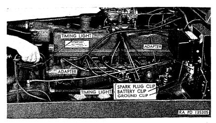
Figure 174. Timing light connected to adapters (installed in ignition circuit).
