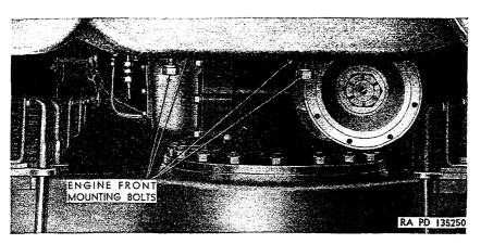
Figure 147. Engine front mounting.
