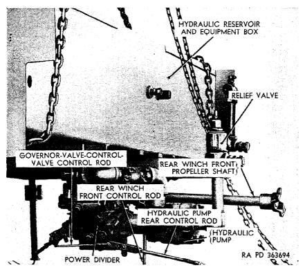
Figure 285. Hydraulic reservoir with power divider, pump, and relief valve removed from vehicle (M62).
