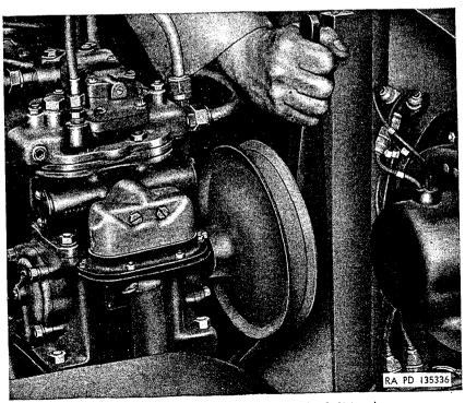
Figure 250. Adjusting air-compressor drive belt tension.
