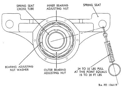
Figure 271. Spring scat bearing adjustment.
