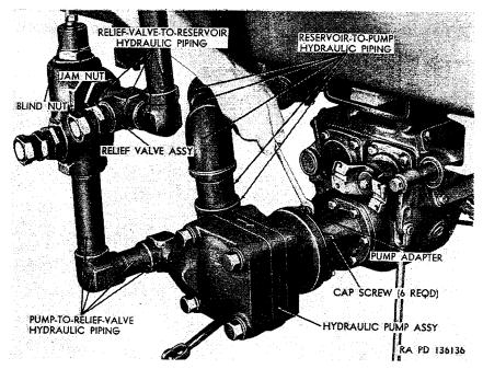
Figure 298. Removing hydraulic pump and relief valve assembly from power divider M62.
