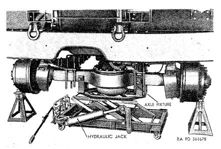
Figure 225. Hydraulic jack positioned for front axle removal.
