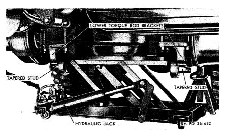
Figure 234. Lower torque rods disconnected.
