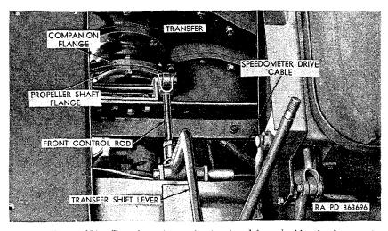
Figure 203. Top view of transfer front end from inside of cab.
