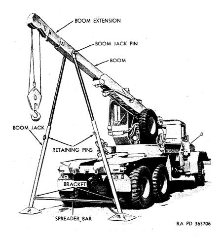
Figure 91. Right rear view of tractor wrecker truck M246 with boom jacks rigged.
