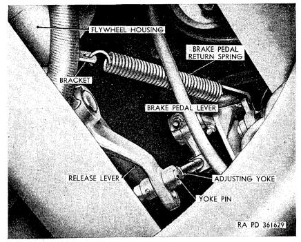
Figure 142. View of clutch linkage from under side of vehicle.
