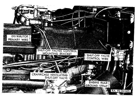
Figure 137. View of upper left side of engine.
