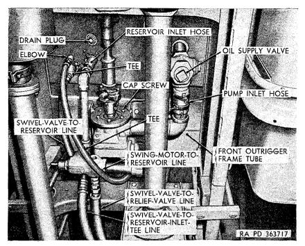
Figure 316. Front bottom view of hydraulic pump and relief valve assembly installed M246.
