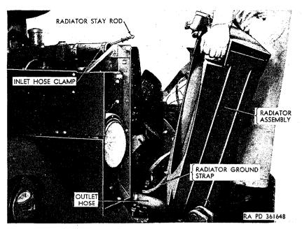
Figure 168. Lifting off radiator assembly.
