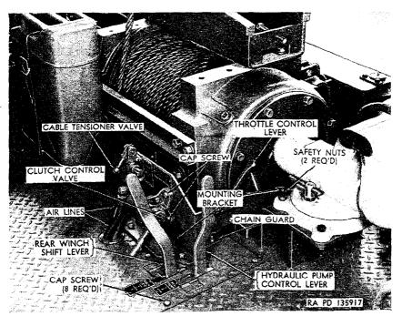
Figure 75. Rear winch controls-M62.
