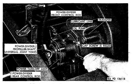
Figure 208. Power-take-off mounted on transfer-M62 only.
