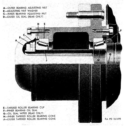
Figure 257. Cutaway view of hub assembly-rear illustrated
