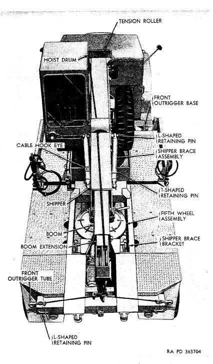
Figure 89. Top rear view of tractor wrecker truck M246.
