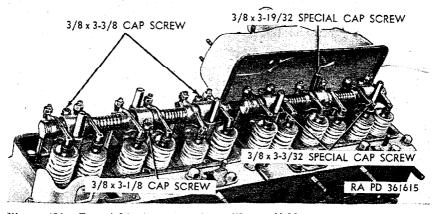
Figure 124. Top right view of engine with manifolds and rocker arm covers removed.
