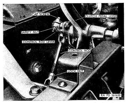
Figure 143. Left front view of clutch pedal lever and control rod. 347797°—55——14
