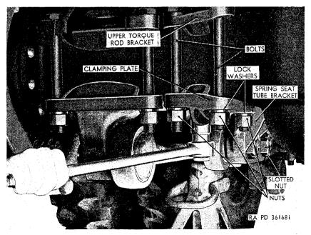
Figure 232. Disconnecting upper torque rod.
