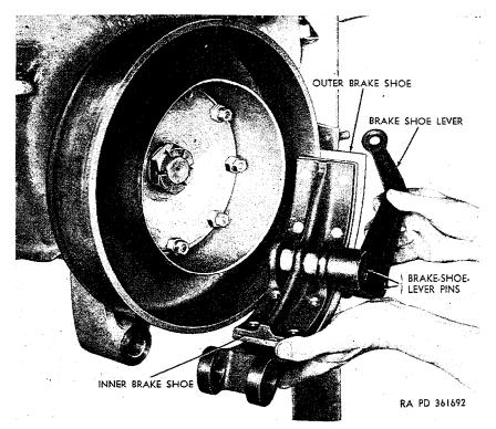
Figure 247. Removing hand brake shoe and lever assembly.
