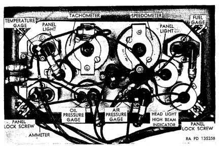
Figure 189. View of back side of instrument cluster.
