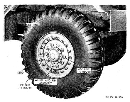
Figure 255. Wheel and tire assembly with bolted-on-type side ring (14:00  $\times$  20 tires)
