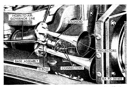
Figure 193. Horn installed on right front fender (solenoid without mounting brackets).
