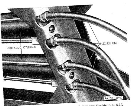
Figure 328. Front bottom view of hoist cylinders and flexible lines M51.
