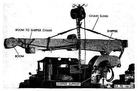
Figure 302. Removing boom and shipper assembly M62.
