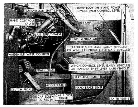
Figure 67. Driver's compartment—left side view.
