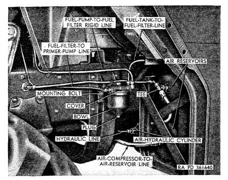
Figure 156.—Fuel filter installed under left front fender.
