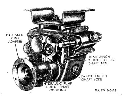
Figure 283. Rear view of power divider removed from vehicle M62.
