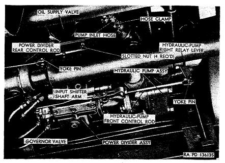
Figure 296. Bottom view of right side of power divider installed M62.
