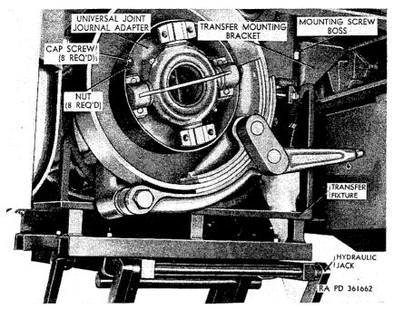
Figure 205. Supporting transfer with hydraulic jack.
