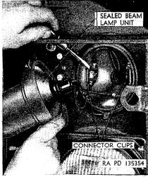
Figure 186. Removing blackout driving light.
