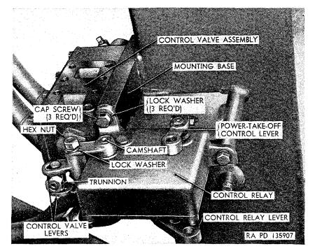
Figure 323. Bottom view of right side of control valve assembly with pump and adapter removed M51.
