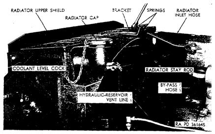
Figure 162. Left rear view of upper section of radiator.
