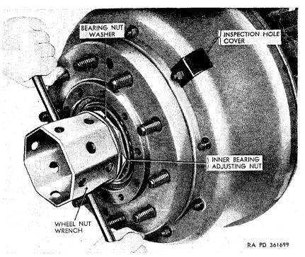
Figure 258. Removing outer bearing adjusting nut.
