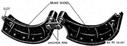
Figure 246. Brake shoes and anchor pins removed from backing plate.
