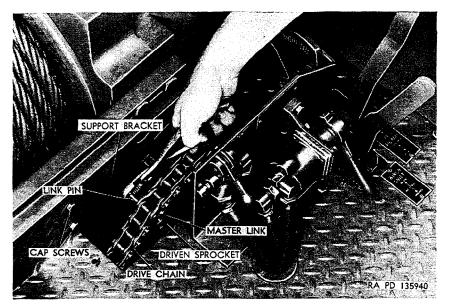
Figure 281. Separating rear winch drive chain M62.
