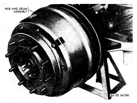
Figure 259. Removing hub and drum assembly.
