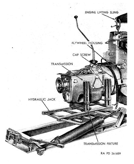
Figure 201. Supporting transmission with hydraulic jack.
