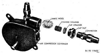
Figure 252. Air-compressor air governor with air strainer disassembled.
