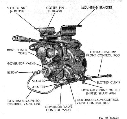
Figure 284. Front view of power divider removed from vehicle M62.
