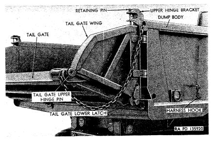
Figure 96. Dump body tailgate arranged for rocker operation.
