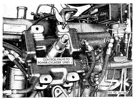
Figure 266. Removing steering gear.
