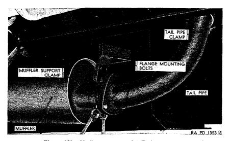
Figure 161. Muffler support and tail pipe mounting.
