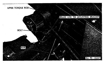
Figure 233. Upper torque rod positioned for forward rear axle removal.
