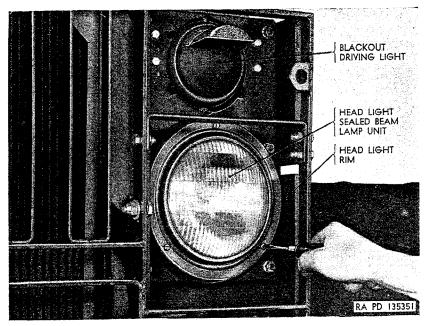
Figure 182. Removing headlight rim.
