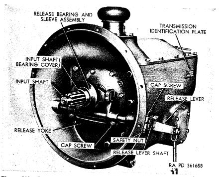
Figure 200. Left front view of transmission and clutch release mechanism.
