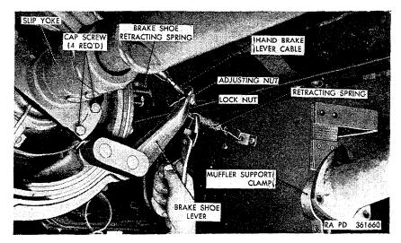
Figure 202. Universal joint and handbrake mechanism at rear of transfer.
