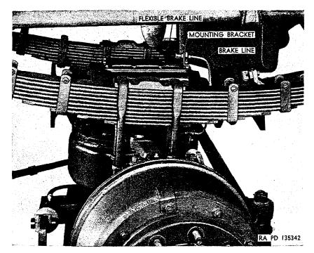
Figure 226. Front axle lowered for disconnecting flexible brake line.
