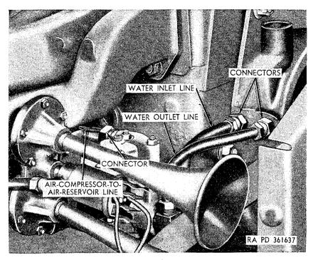
Figure 153. Air compressor lines and connectors.
