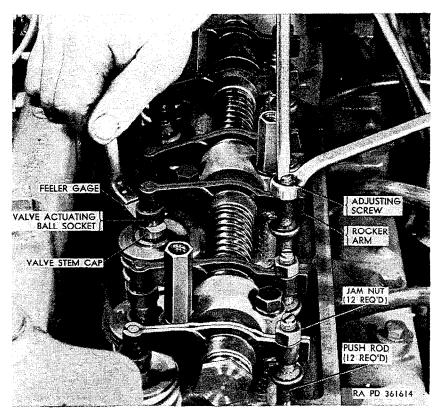
Figure 123. Adjusting valve clearance.
