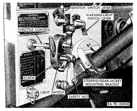
Figure 72. Throttle control in LOCKED-OUT position.
