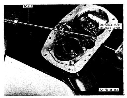
Figure 177. Checking distributor breaker lever spring tension.
