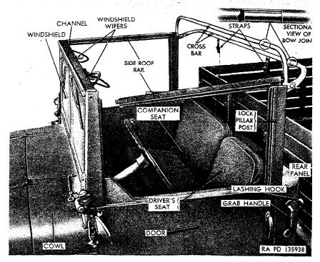
Figure 334. Top left view of cab with top paulin removed.
