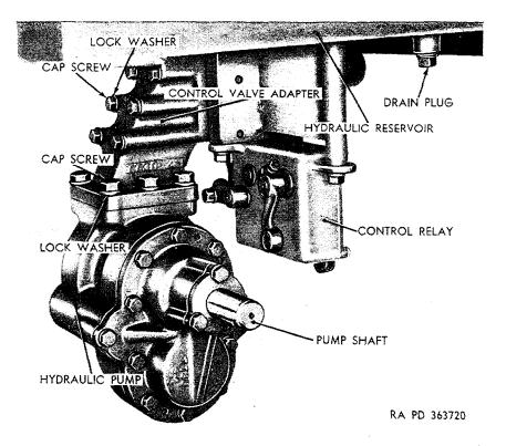
Figure 322. Right front view of hydraulic hoist pump mounting M51. .
