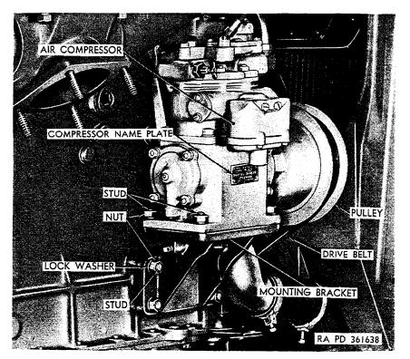
Figure 154. Air compressor mounting.
