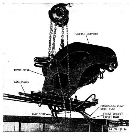
Figure 299. Removing base plate and pivot post assembly from crane body M62.
