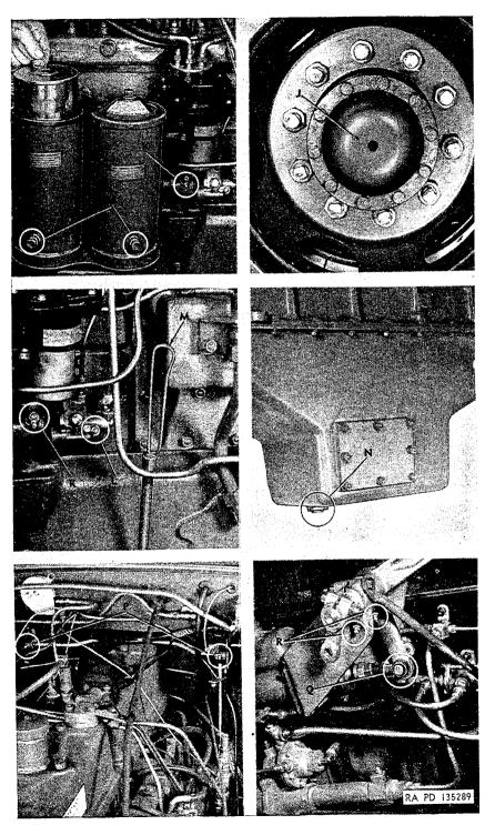
Figure 108. Localized lubrication points (H-R).
