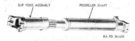
Figure 214. Propeller shaft assembly.
