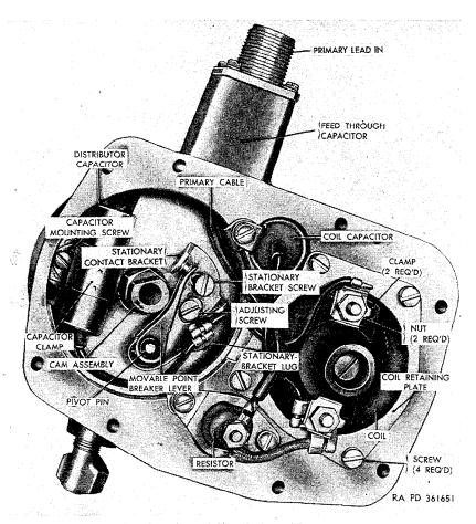
Figure 176. Top view of distributor with cover removed.
