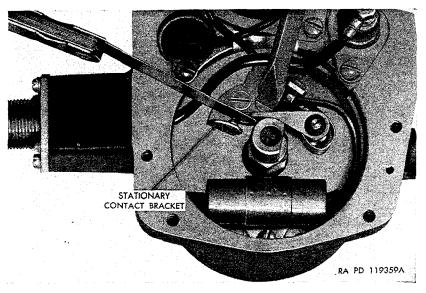
Figure 178. Checking and setting distributor contact point gap.
