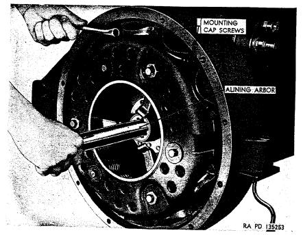
Figure 199. Using alining arbor to install clutch.
