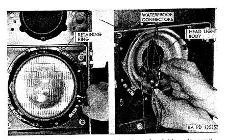
Figure 183. Removing headlight retaining ring and scaled-beam lamp-unit.
