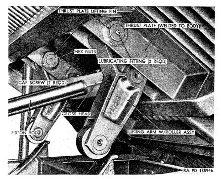
Figure 325. Left side of hoist assembly with dump body in raised position M51.
