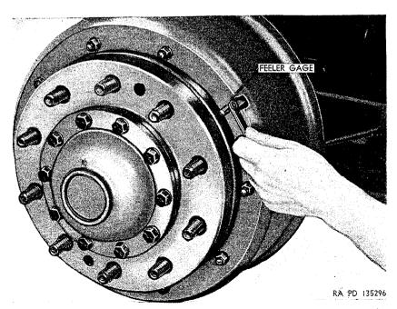
Figure 242. Checking clearance between brake shoe and drum.
