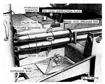
Figure 90. View of right front section of wrecker body-M246.
