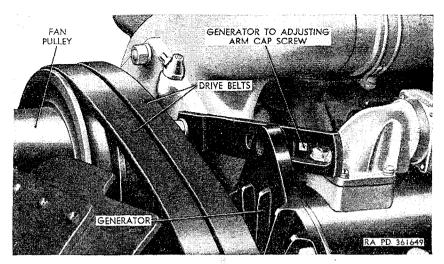
Figure 164. Drive belts installed on fan pulley.
