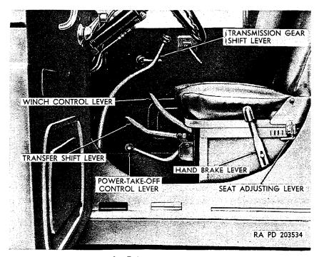
Figure 68. Driver's compartment—M246.
