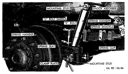
Figure 270. Left front spring and shock absorber—installed.
