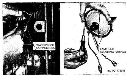
Figure 187. Removing sealed-beam,
