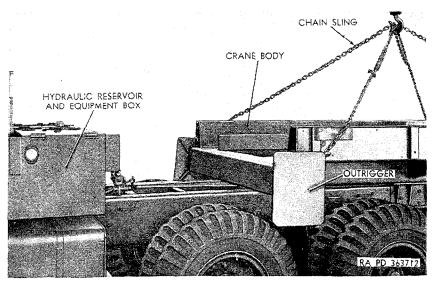
Figure 311. Removing crane body M62.
