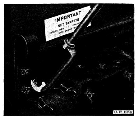
Figure 172. Removing spark plug cable.
