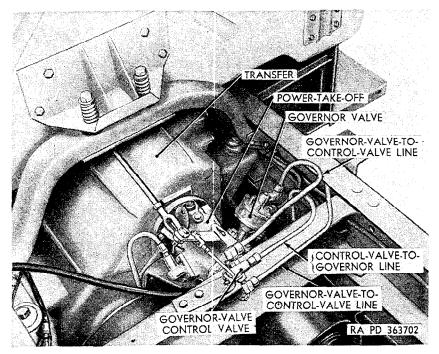
Figure 87. Power-take-off mounted on rear of transfer (M246 only)—top left rear view.
