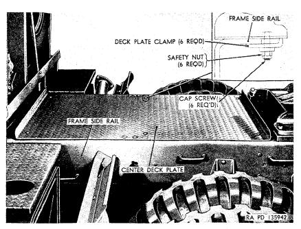
Figure 321. Top left view of center deck plate M52.
