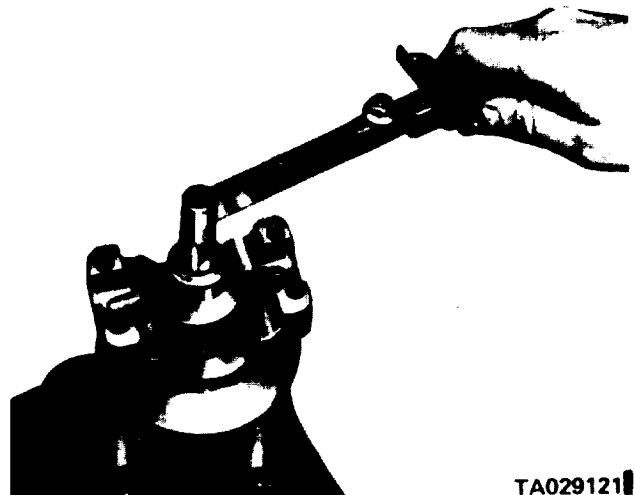
Figure 20-15. Checking Pinion Bearing Preload.
