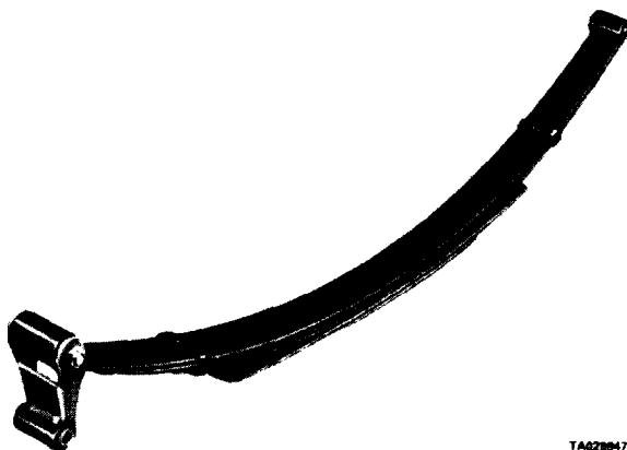
Figure 7-8. Progressive Type Spring.
