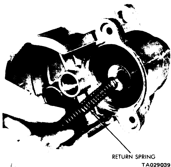
Figure 15-12. Removing Return Spring.
