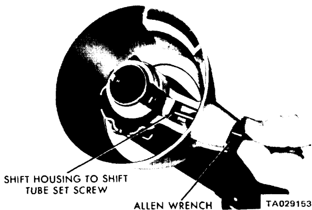
Figure 21-15. Shift Tube Set Screw.
