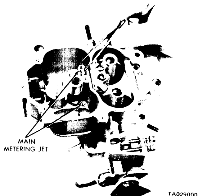
Figure 12-7. Removing or Installing the Main Metering Jets.
