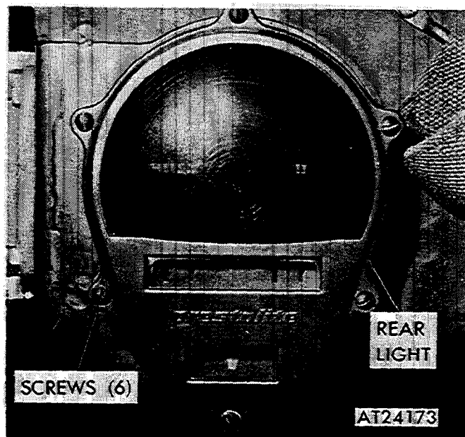
Figure 2-210. Removing or installing door to rear light housing (M151A2, M825, and M718A1 vehicles).
