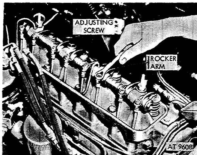
Figure 2-61. Back off adjusting screws.
