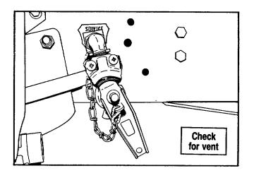
3. That's because the service dummy coupling needs a breather vent to release air pressure. If you have the right coupling and the brakes lock up, the vent hole may be plugged with dirt or paint.
