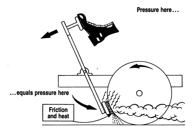
c. Hydraulic and air/hydraulic brakes work because of a simple law of hydraulics; pressure cannot compress fluid, but fluid will transfer pressure.
