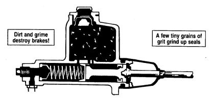
3. Grit and dirt usually sneak into the brake system when you check or add fluid. This is true for all vehicles, but the problem is worse on 2 1/2- and 5-ton trucks. Dirt has more chances to get into the brake system because the master cylinder is located underneath the trap door in the floorboard..
