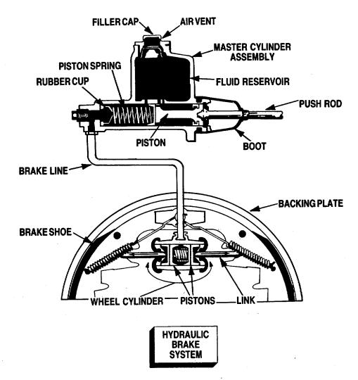
b. When brake shoes press hard against a drum or rotor, they develop friction. This friction does-the braking. The truck stops as long as you have good brake linings and an airtight hydraulic system filled with fluid.
