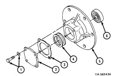
FRAME 7 NOTE Do not take out two lower screws from support tube in step 1. Take out four nuts, lockwashers and two upper screws (1) holding support 1. tube (2) to brake shell (3). 2. Take out two screws and washers (4). CAUTION Be careful when taking out drive gear from clutch case (5). They can easily be damaged. 3. Slide clutch case (5) and housing assembly (6) off drive clutch and brake assembly (7) using hoist. GO TO FRAME 8 4 TA 085438
