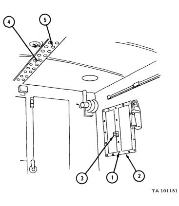
FRAME 2 Take out two screws (1). 1. Take out two nuts (2) and take off blower bracket (3). 2. 3. Take out eight screws (4). Take off blower assembly (5). 4. GO TO FRAME 3 1 3 2 808 808 Π П 5 4 TA 101182
