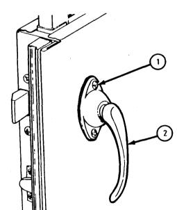
FRAME 2 Take out screw (1). Take off inner door handle (2) and washer (3). 1. Take out six screws (4) and take off inspection hole cover (5). 2. GO TO FRAME 3  $\widehat{\mathbf{1}}$ 00 4 5 TA 104878
