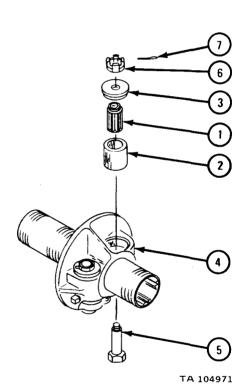
FRAME 5 NOTE Shims (1) must be the same thickness as noted in removal. Put on shims (1). 1. Pack upper tapered roller bearing (2) with grease. Put on roller bearing. 2. GO TO FRAME 6 (2)TA 104972
