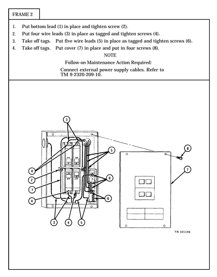
17-37. CONVERTER REMOVAL AND REPLACEMENT (TRUCKS M109A2 AND M109A3). TOOLS: No special tools required SUPPLIES: None PERSONNEL: Two EQUIPMENT CONDITION: Truck parked, engine off, handbrake set. a. <u>Removal.</u>
