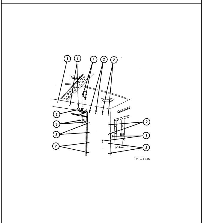
FRAME 3 Soldiers 1. Put up left rear ceiling panel (1). Aand B Soldier B 2. Hold left rear ceiling panel (1) up. Soldier A 3. Put in 15 screws (2). GO TO FRAME 4
