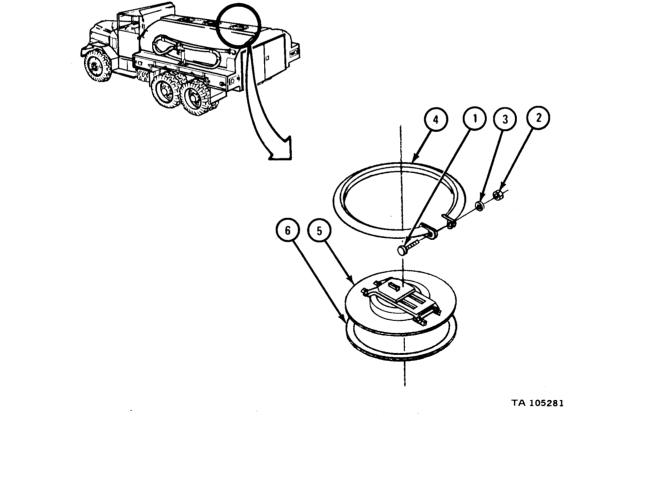
FRAME 2 Soldier A 1. Hold nut (1). Soldier B 2. Unscrew coupling nut (2). Soldier A 3. Take out nozzle (3). Soldiers 4. Take off discharge hose (4). A and B Soldier A 5. Hold two nuts (5). Soldier B 6. Take out two screws(6). 7. Take off nozzle bracket (7). GO TO FRAME 3 3 2 6 2 5 TA 105282
