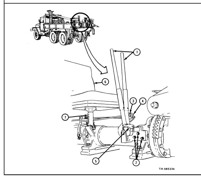
17-53. POWER LEVELER REMOVAL, REPAIR, AND REPLACEMENT (TRUCK M764). TOOLS: No special tools required.
