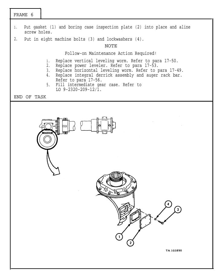
17-48. MAIN DRIVE IDLER GEAR ASSEMBLY REMOVAL, REPAIR, AND REPLACEMENT (TRUCK M764).
