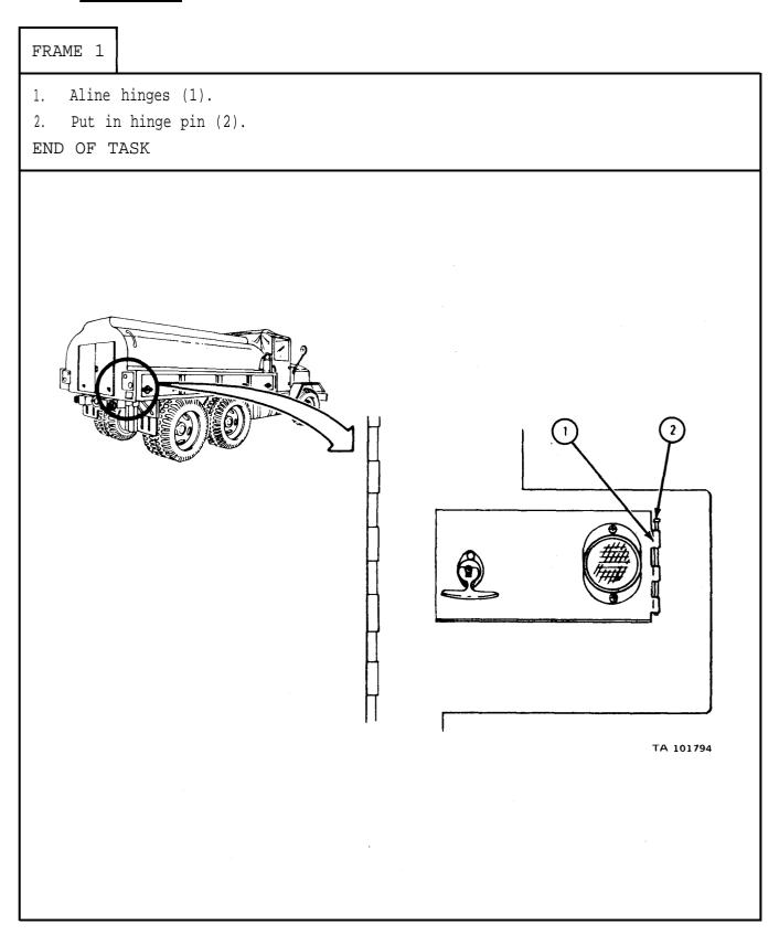
17-21. TANK BODY DOOR HOLDER REMOVAL, REPAIR, REPLACEMENT, AND ADJUSTMENT.
