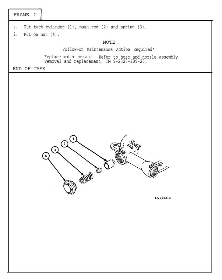
17-33. WATER DISCHARGE PIPE REPAIR (TRUCKS M50A2 AND M50A3).
