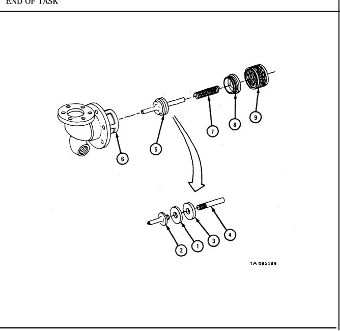
17-26. CENTRIFUGAL PUMP REPAIR (TRUCKS M49A1C, M49A2C, M50A1, M50A2, AND M50A3).
