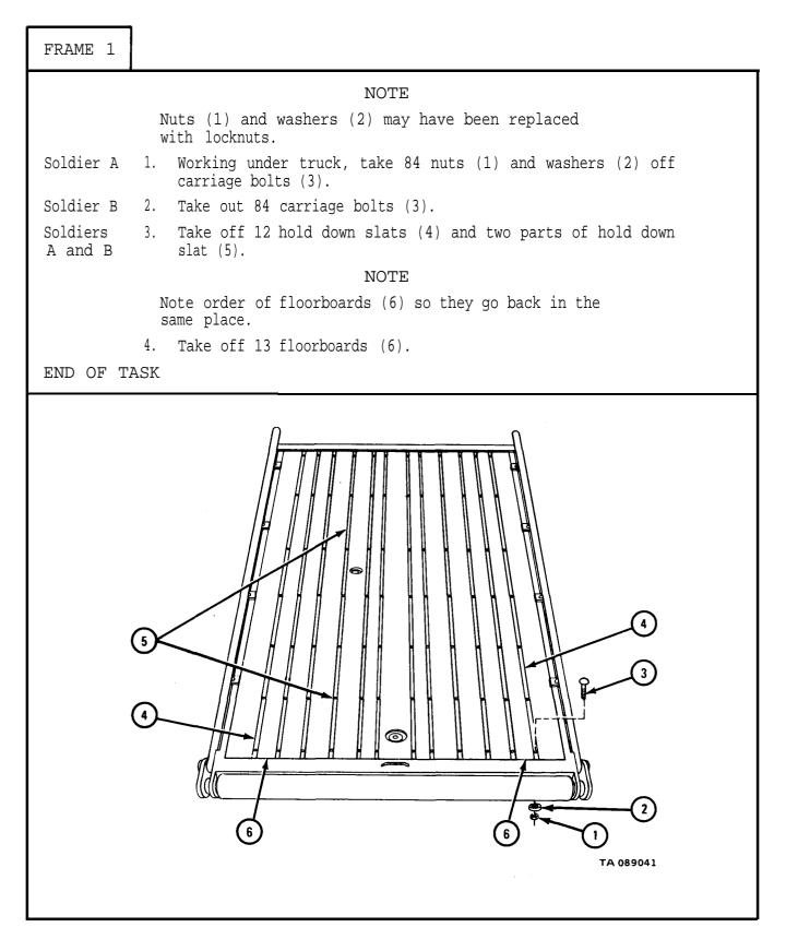
c. Cleaning. Clean hold down slats and floorboards with soapy water and rags. Let parts air dry.
