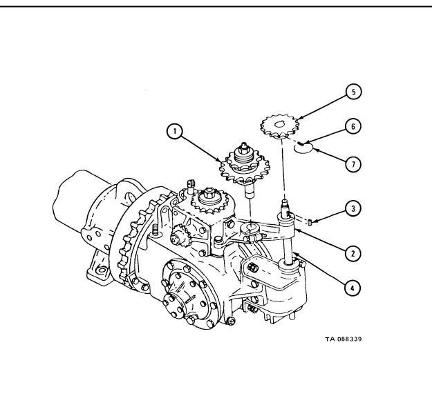
17-51. OPERATION LEVER ASSEMBLY REMOVAL, REPAIR, AND REPLACEMENT (TRUCK M764). TOOLS: No special tools required SUPPLIES: Cotter pin (2) PERSONNEL: One EQUIPMENT CONDITION: Truck parked, engine off, handbrake set. a. Removal.
