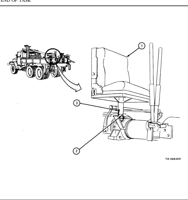
17-45. EARTH BORING MACHINE ASSEMBLY REMOVAL AND REPLACEMENT. TOOLS: No special tools required SUPPLIES: Wood blocks PERSONNEL: Т₩О EQUIPMENT CONDITION: Truck parked, engine off, handbrake set.
