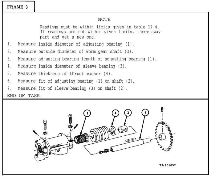
Table 17-4. Adjusting Bearing, Wormgear Shaft, and Thrust Washer Wear Limits
