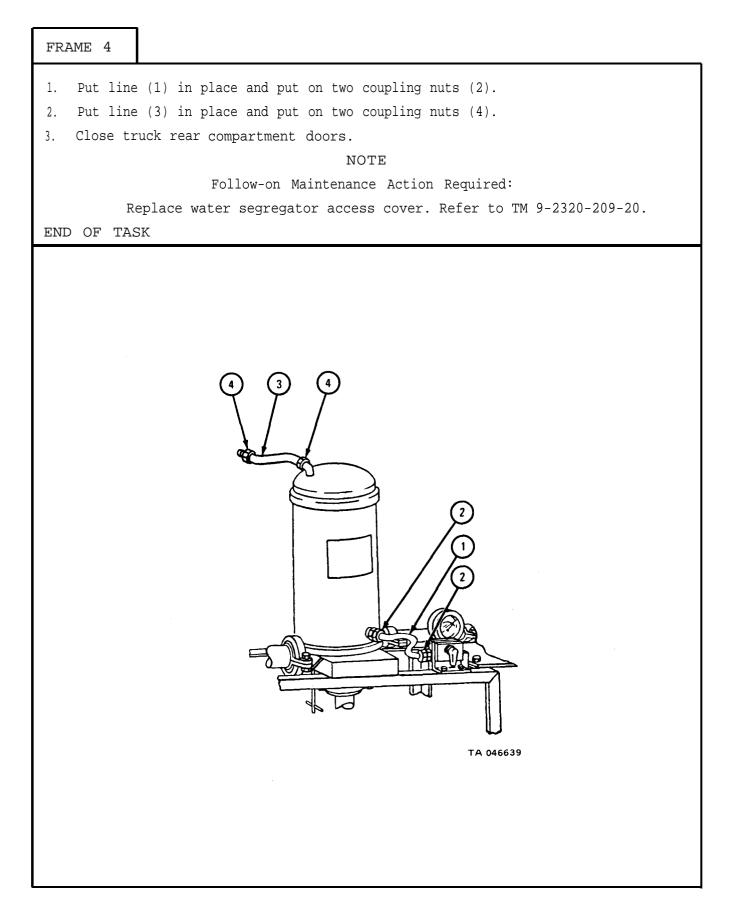
17-23. WATER SEGREGATOR FILTER REMOVAL, REPAIR, AND REPLACEMENT (TRUCK M49A2C).
