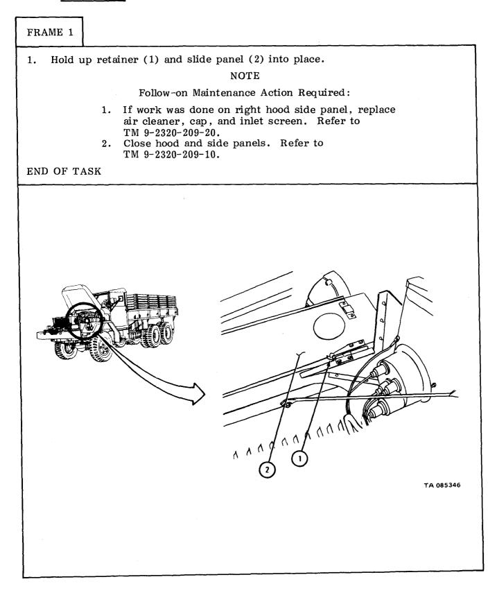
17-4. HOOD ASSEMBLY REMOVAL, REPAIR AND REPLACEMENT. TOOLS: No special tools required SUPPLIES: Solvent, dry cleaning, type II (SD-2), Fed. Spec P-D-680 PERSONNEL: Two EQUIPMENT CONDITION: Truck parked, engine off, handbrake set.
