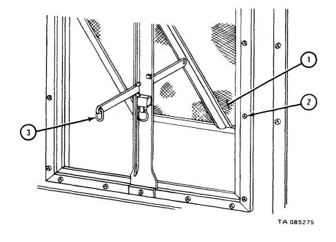
17-41. LIFTING SHACKLE REMOVAL, REPAIR, AND REPLACEMENT (TRUCKS M109A2, M109A3, M185A2, AND M185A3).
