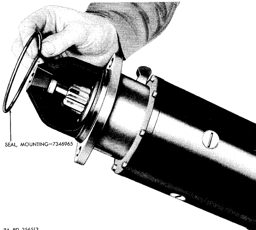
Figure 98. Installing mounting seal on starter housing.
