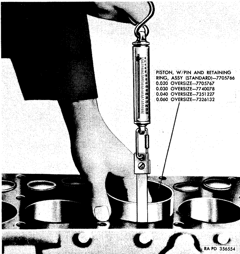
Figure 61. Fitting piston to rebored cylinder.
