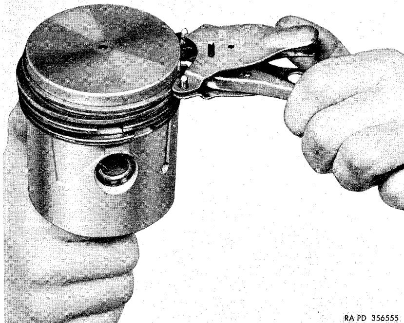
Figure 62. Installing piston rings with piston ring applicator 41-A-329-500.
