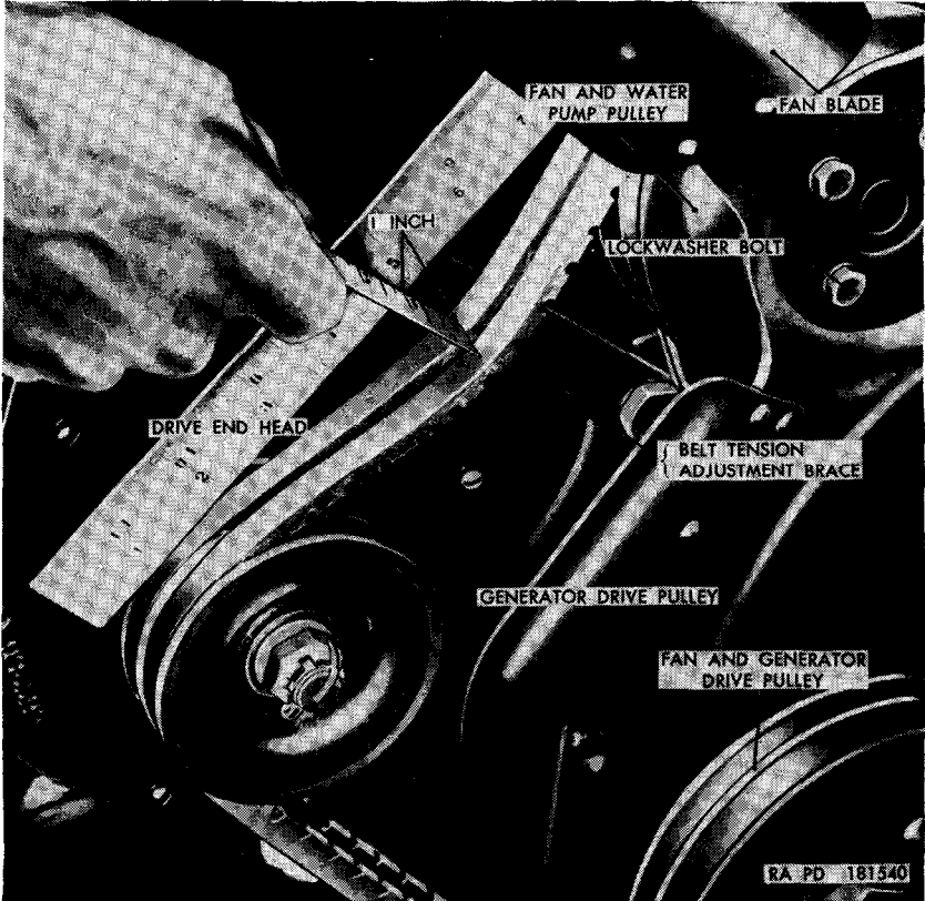
Figure 42. Adjusting drive belts.
