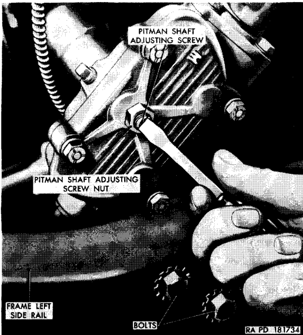
Figure 112. Adjusting steering gear.
