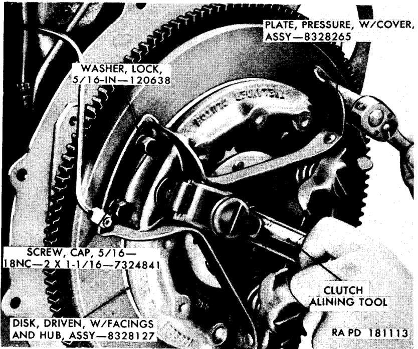
Figure 102. Installing clutch pressure plate w/cover assembly.
