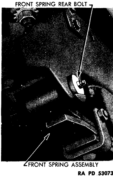
Figure 196—Front Spring Rear Bolt
