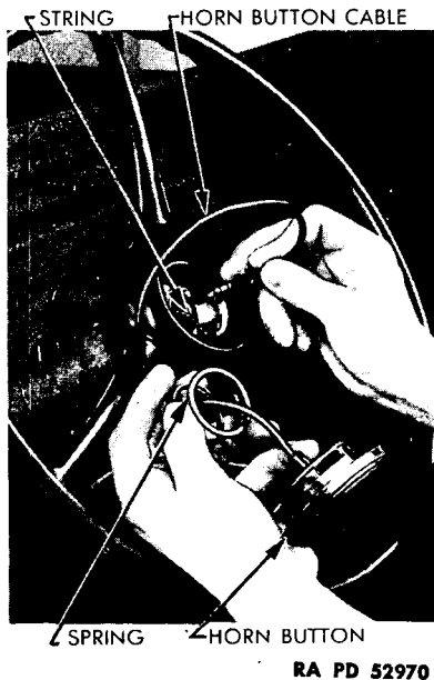
Figure 133—Installing Horn Button Cable
