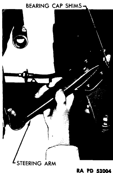
Figure 161—Removing Steering Arm
