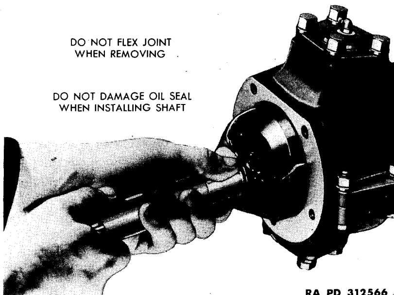
Figure 157—Removing Universal Drive Assembly
