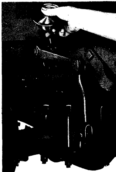
Figure 200—Filling Shock Absorber with Fluid
