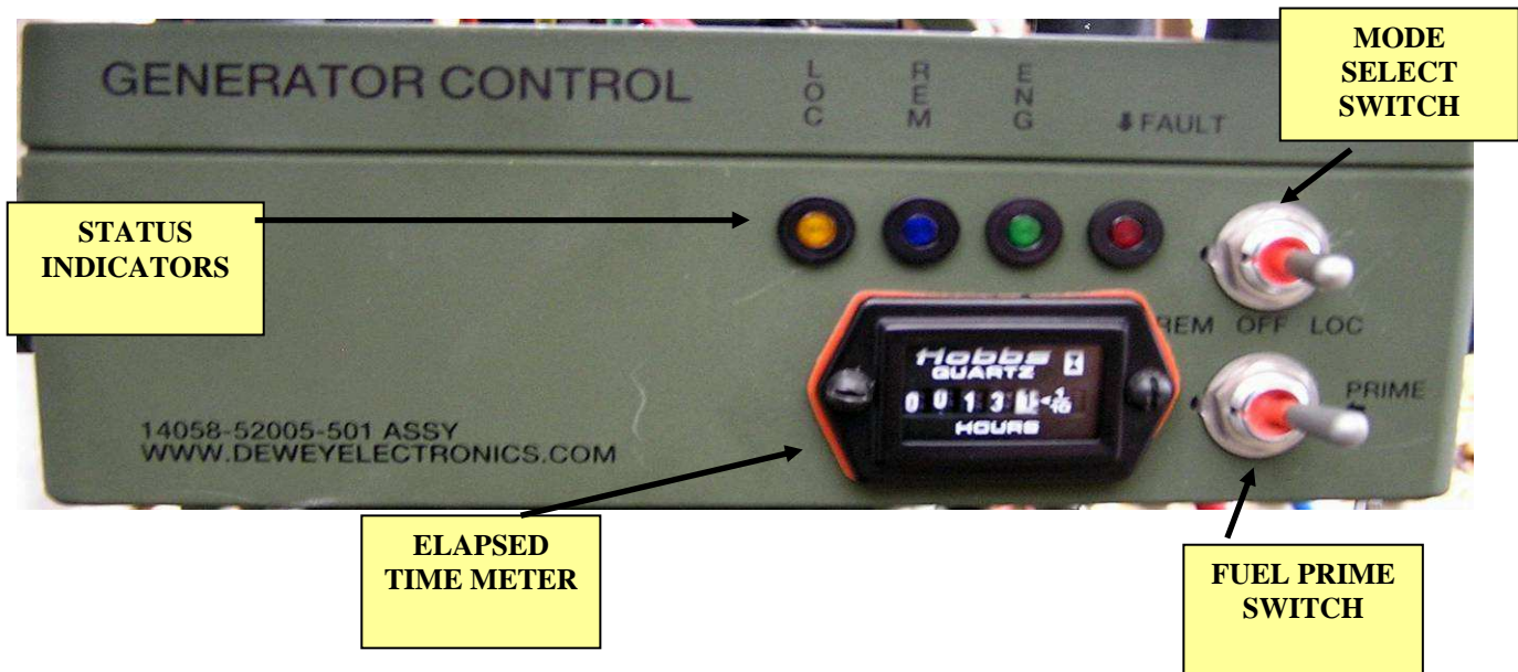
FIGURE 2 VPS – GENERATOR CONTROLLER
