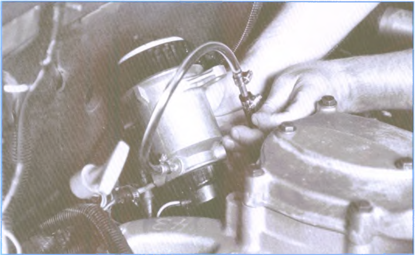
Figure 7-68, Check for Air in Fuel at Injection Pump Inlet
