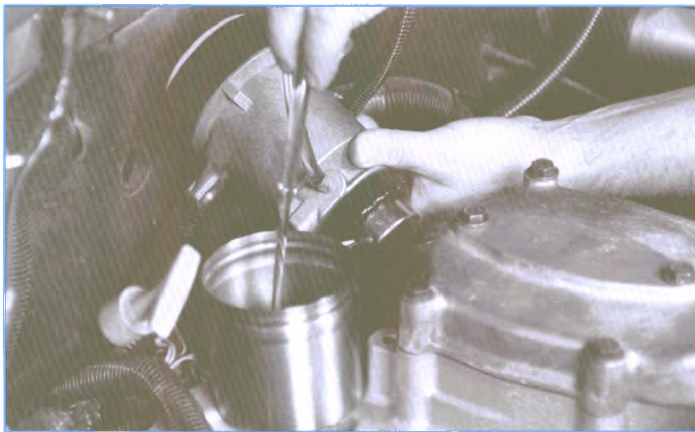
Figure 7-66, Volume Check at Fuel Filter Outlet
