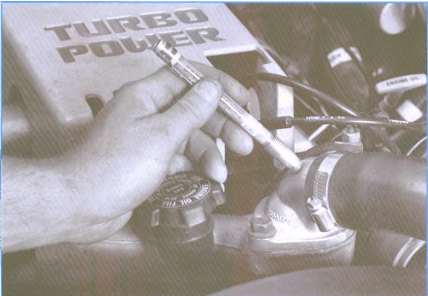
Figure 4-17, Cooling System Thermostat Diagnosis
