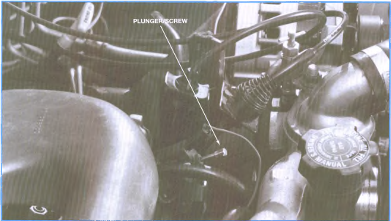
Figure 7-81, Idle Speed Adjustment (2)
