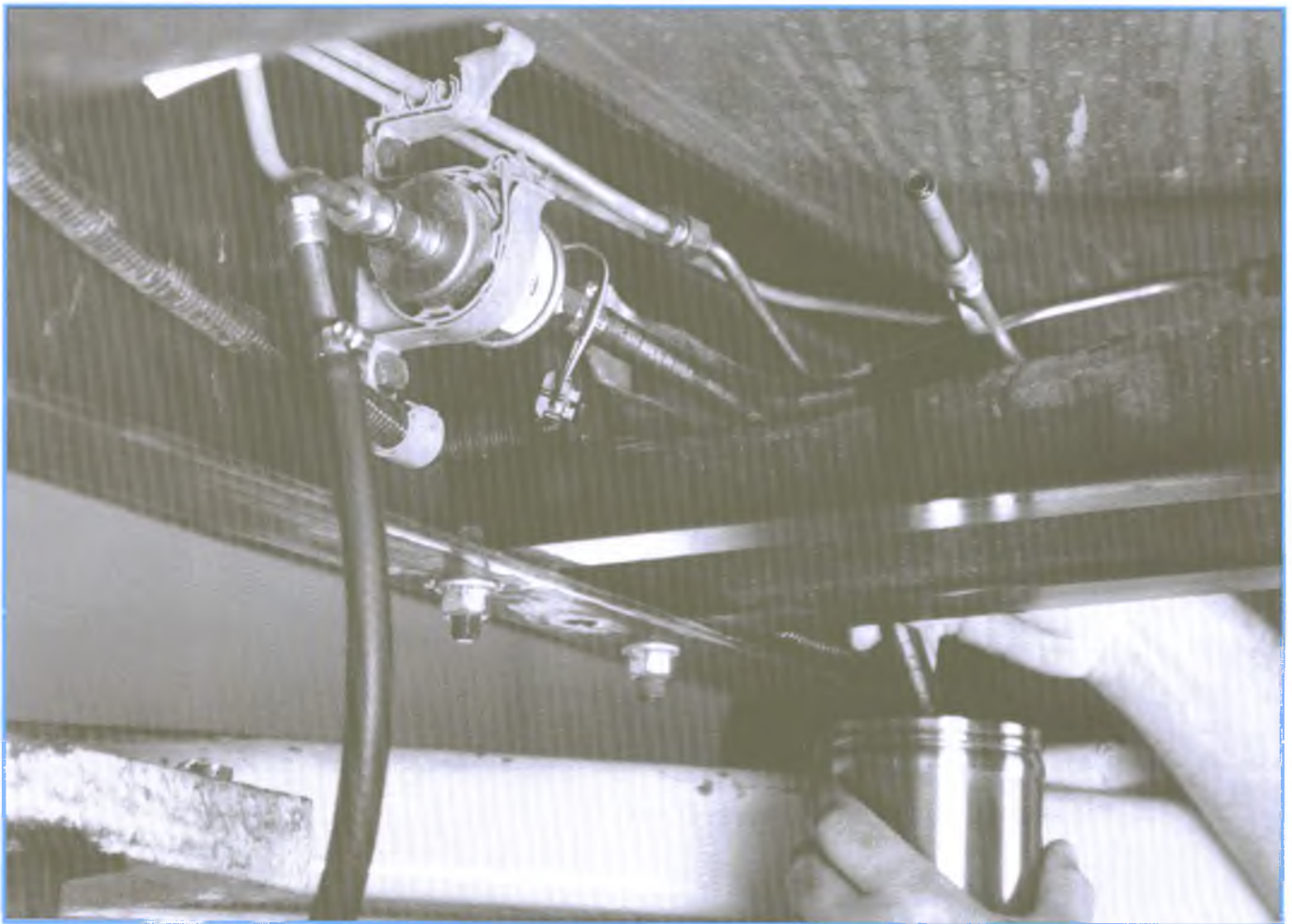
Figure 7-63, Volume Check at Lift Pump Outlet (2)
