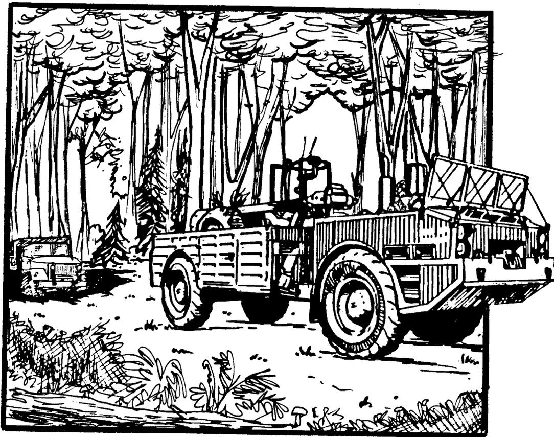
Place the wrecker in the recovery position. Here the disabled mired vehicle is an M817 5-ton dump truck.
