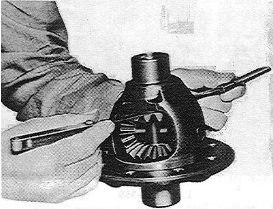
Figure 13-19. Checking side gear clearance.
