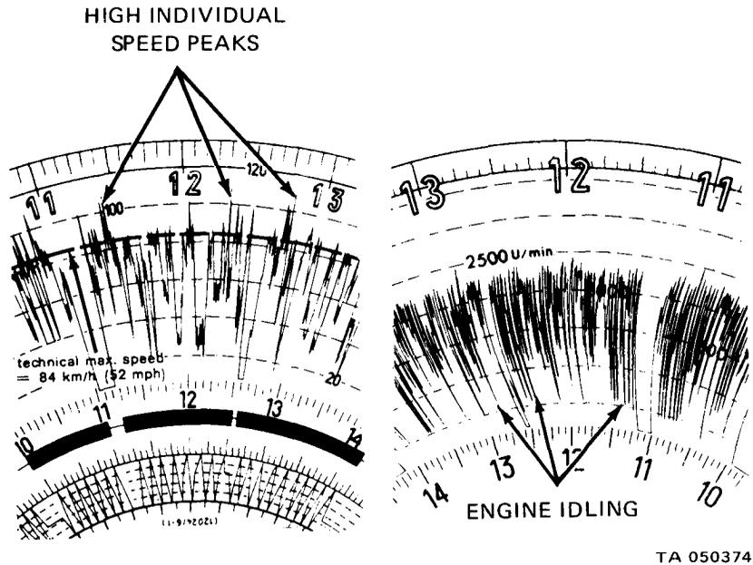
Figure 20-10. Driving Downhill without Gear Engaged
