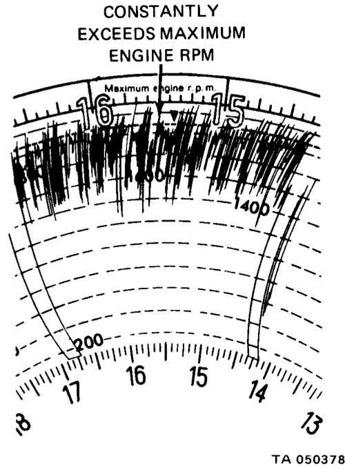
Figure 20-14. Engine Run at Excessively High RPM
