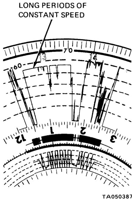
Figure 20-23. Speed Recording Runs for Unusually Long Period at a Uniform Level
