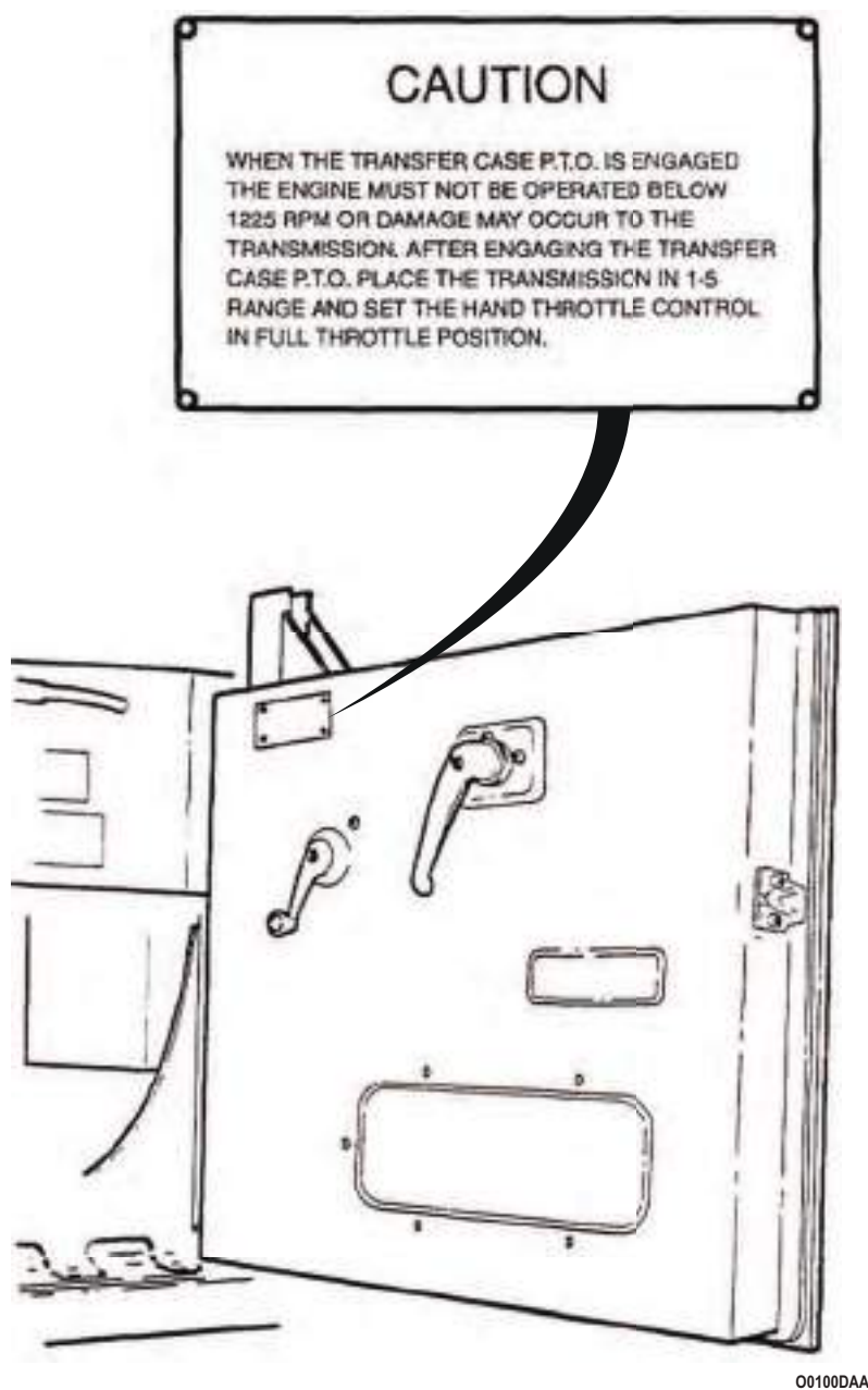
Figure 21. Transfer Case PTO Caution Decal.
