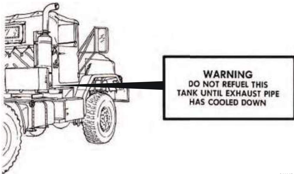
Figure 12. Fueling Warning Decal.
