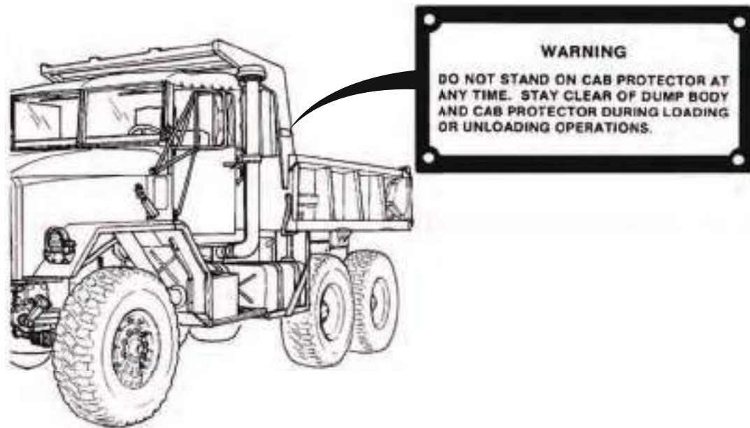
Figure 14. Dump Bed Warning Decal.
