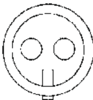
Figure 1. Wheel Speed Sensor Connector.
