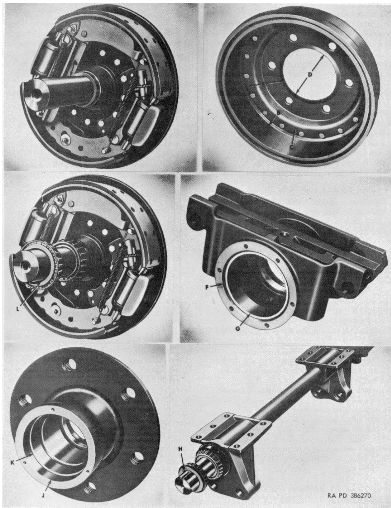
Figure 6-1. Standard repair measurement points
