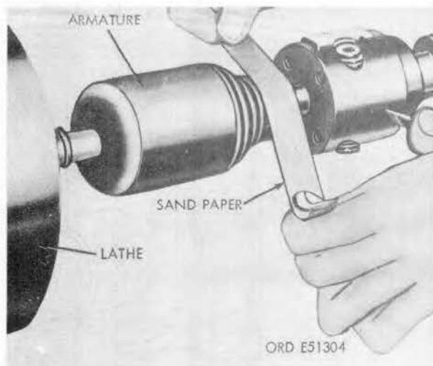
FIGURE 29. SMOOTHING BURS WITH NO. 00 SANDPAPER.
