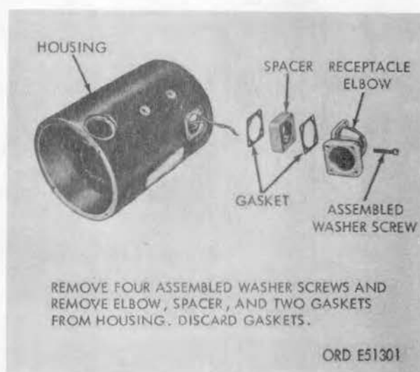
FIGURE 19. REMOVING RECEPTACLE ELBOW.
