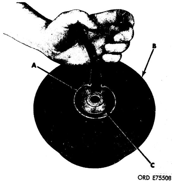
Figure 70. Removing compressor insert retaining snap ring.
