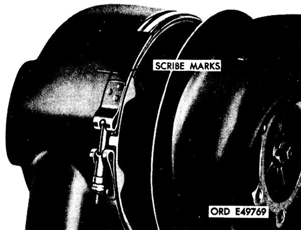
FIGURE 14. SCRIBING ALINEMENT MARKS ON COMPRESSOR COVER AND BEARING HOUSING - TURBOCHARGERS 10935279, 10912638, AND 53591-C-139552.
