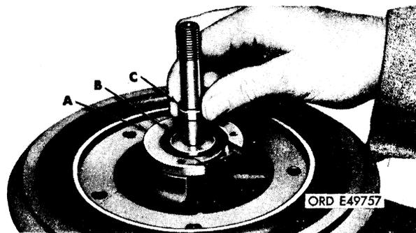
FIGURE 48. PLACING REAR OIL RETAINER, THRUST RING, AND SPACER SLEEVE OVER BEARING HOUSING - TURBOCHARGERS 10912638 AND 53591-C-139552.
