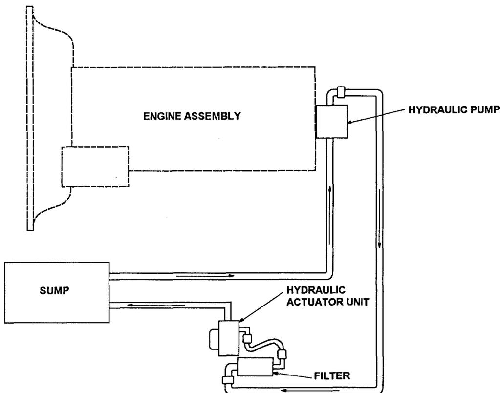
**Figure 1-12. Hydraulic System Diagram
