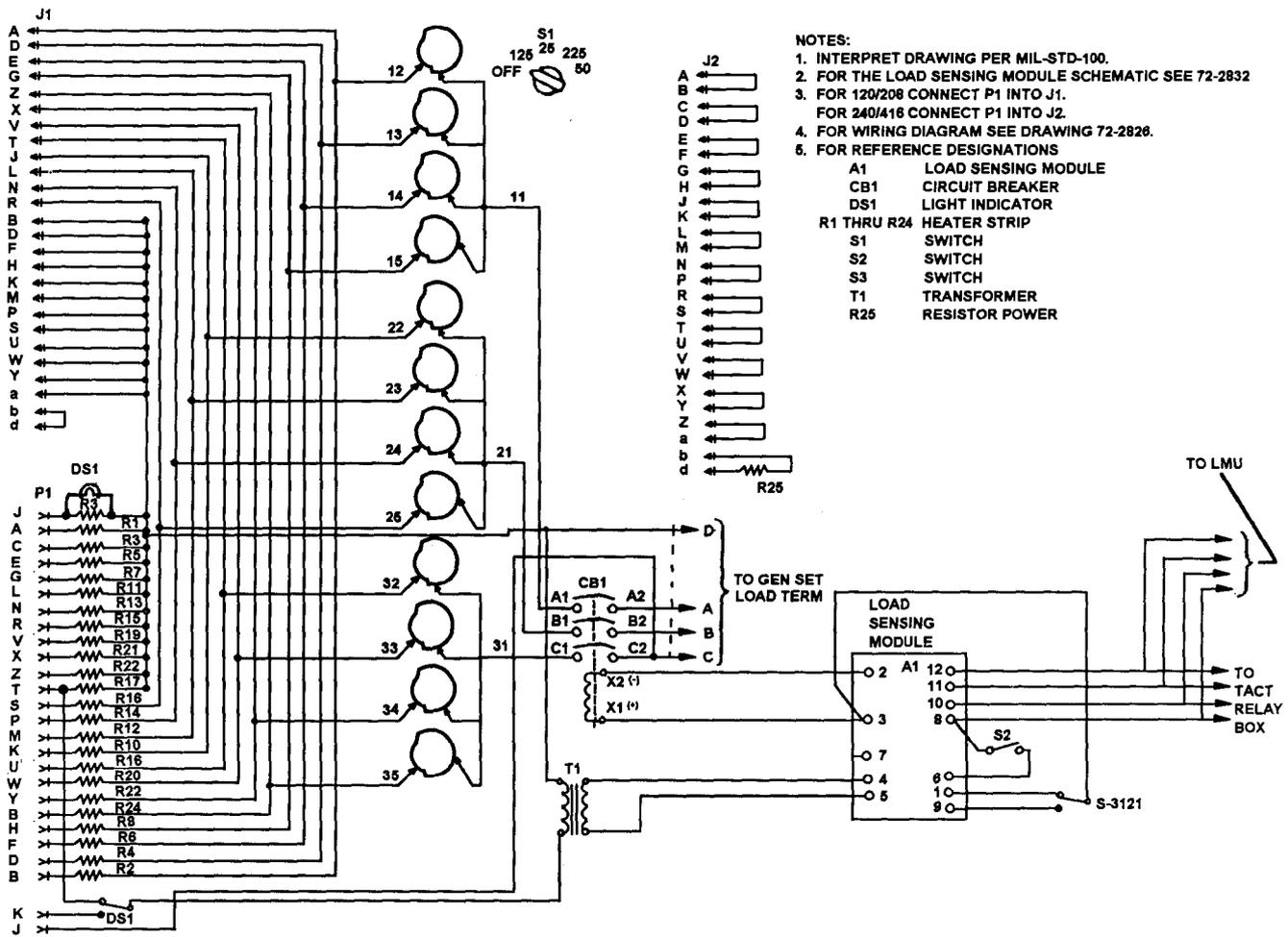
Figure 5-14. Load Bank Schematic Diagram, Dwg. No. 72-2827
