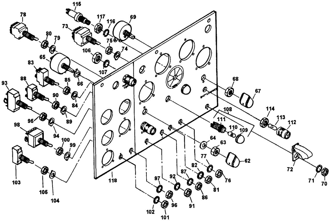
Figure 4-38. Control Cubicle Assembly, Exploded View (Sheet 2 of 3)
