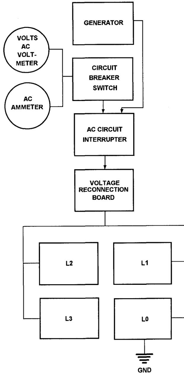
Figure 1-11. Output Supply System
