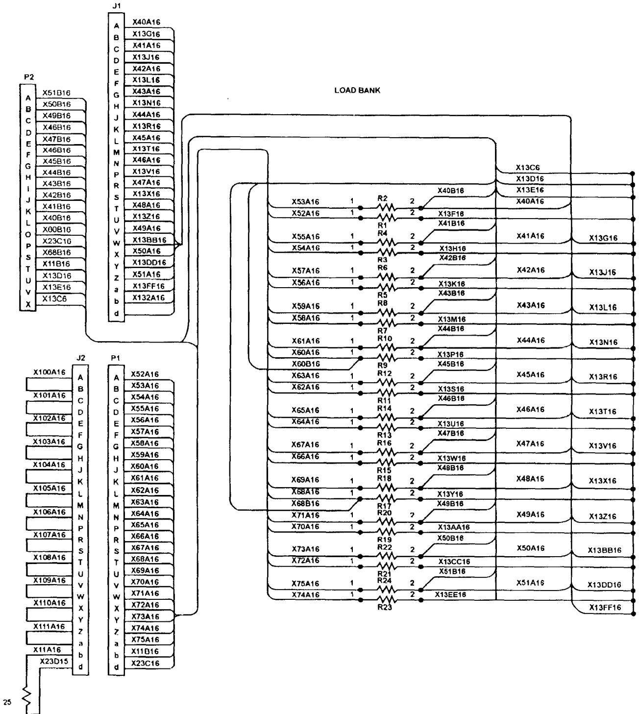
Figure 5-13. Load Bank Wiring Diagram, Dwg. No. 72-2826 (Sheet 2 of 2)
