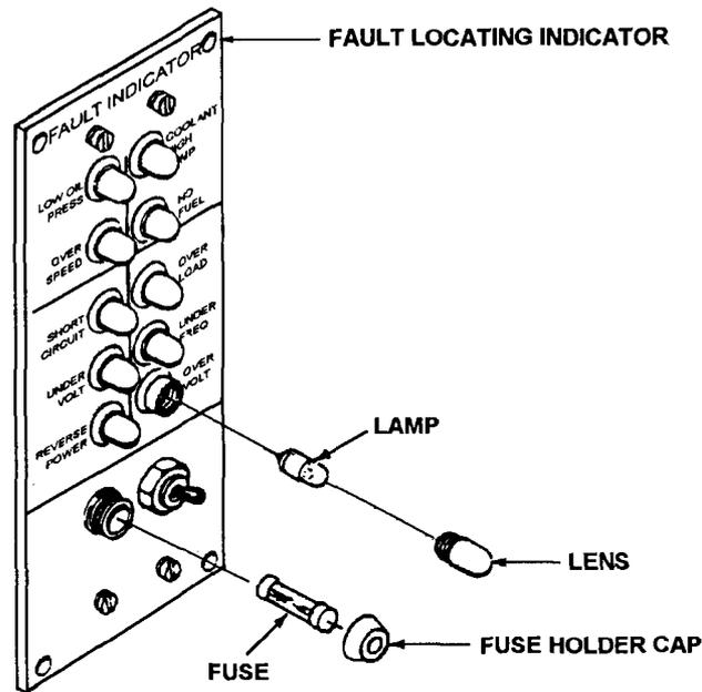
**Figure 4-40. Fault Locating Indicator Lamp and Fuse Replacement**
