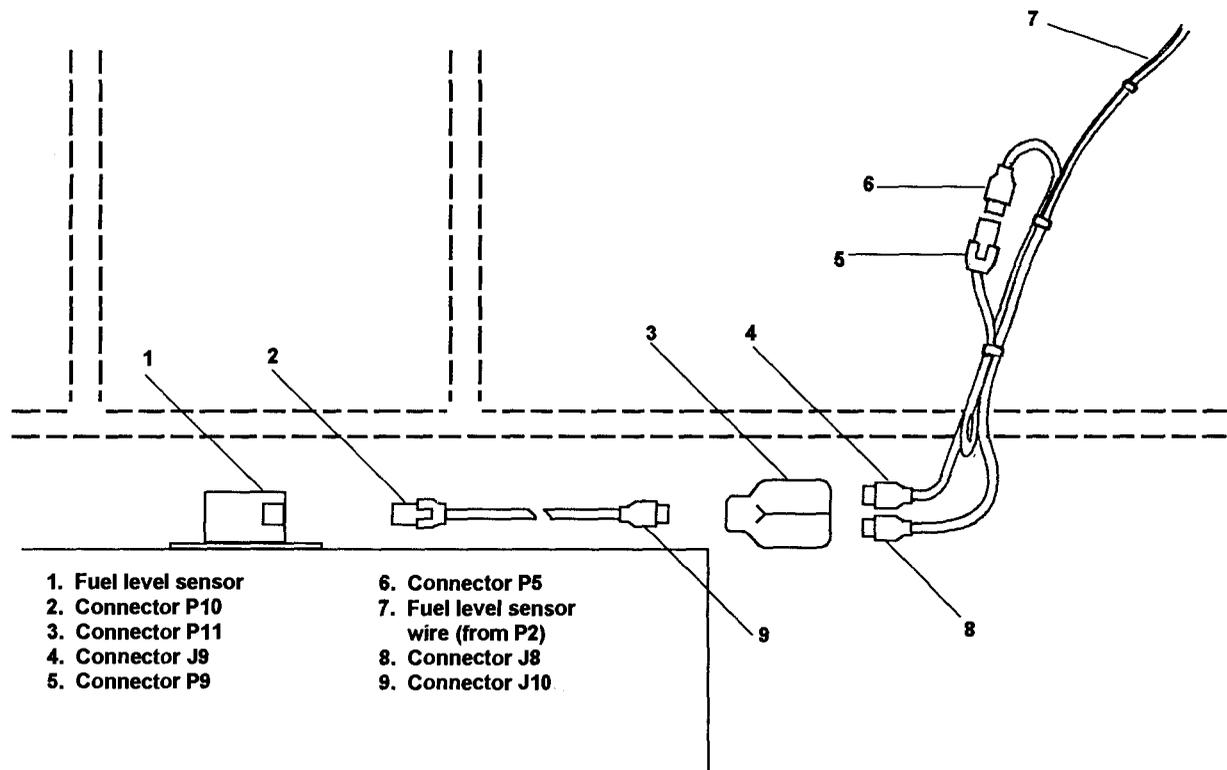
Figure 5-17. Applications Kit Cable Harness Assembly Installation (Left Side)
