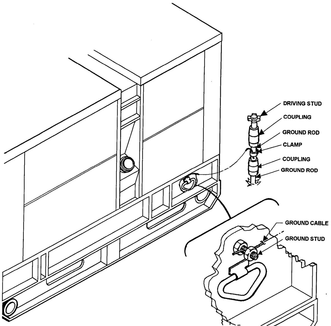
Figure 2-3. Ground Connections
