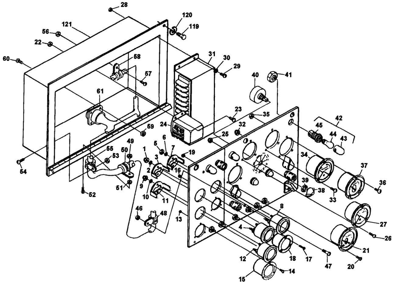
Figure 4-38. Control Cubicle Assembly, Exploded View (Sheet 1 of 3)
