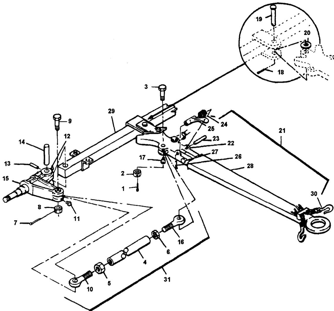
Figure 5-9. Wheel Mounting Kit, Front Axle and Tow Bar Assembly, Exploded View
