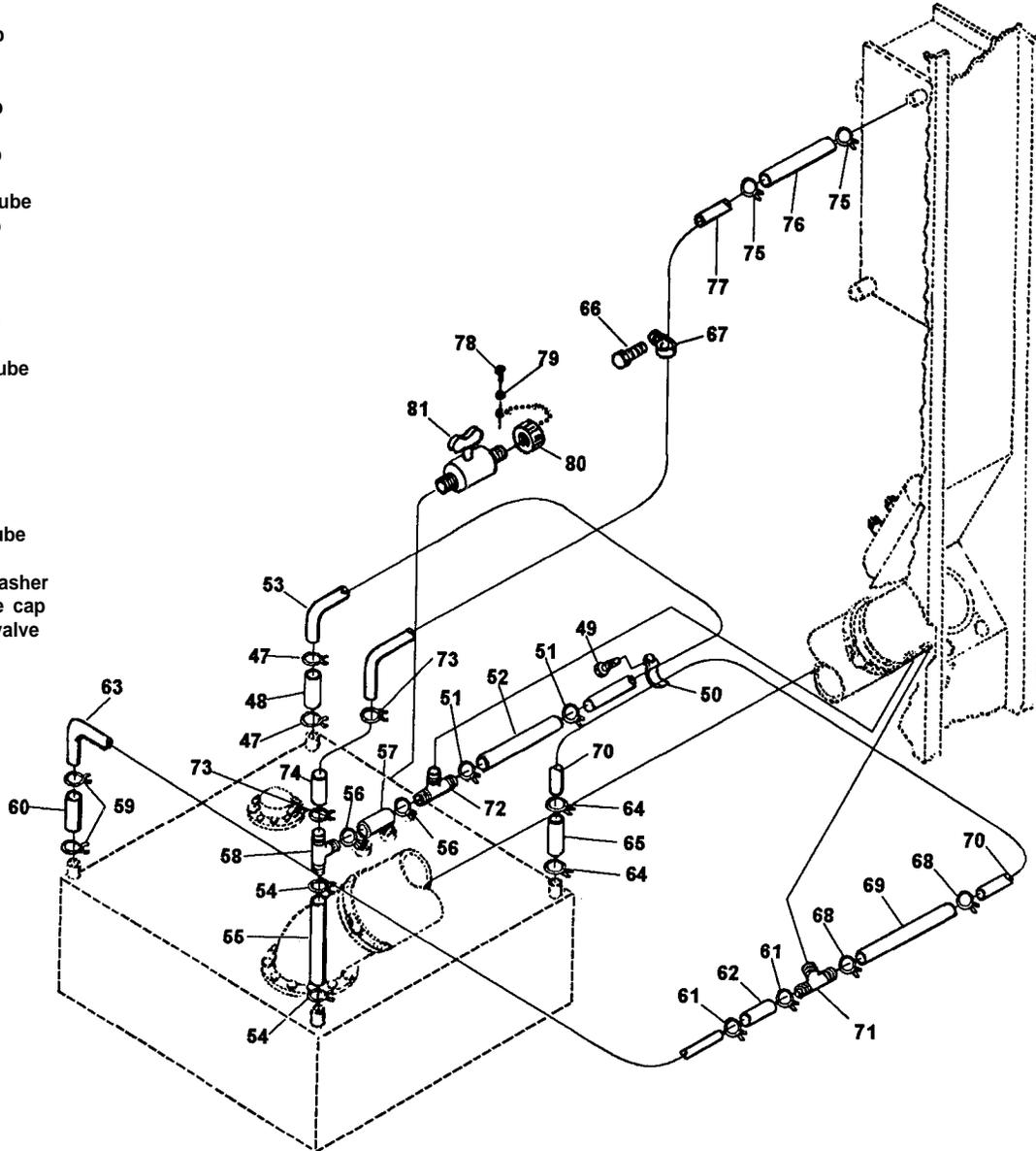
Figure 4-21. Fuel Lines and Fittings, Exploded View (Sheet 2 of 2)
