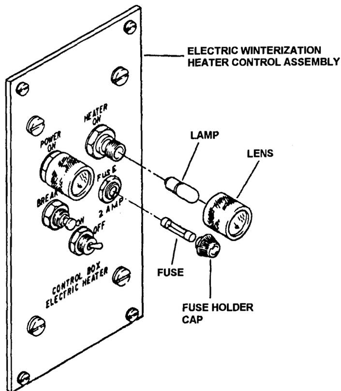
Figure 5-6. Electric Winterization it Control Assembly Indicator Lamp Fuse Replacement
