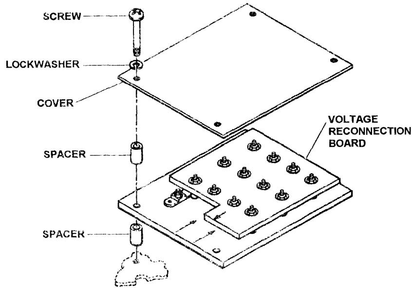
**Figure 4-45. Voltage Reconnection Board, Removal and Installation**
