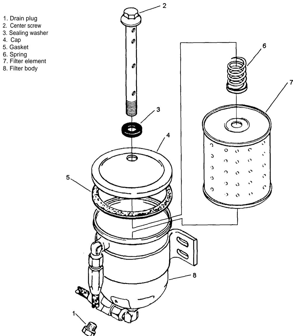
**Figure 4-1. Servicing the Engine Oil Filter**
