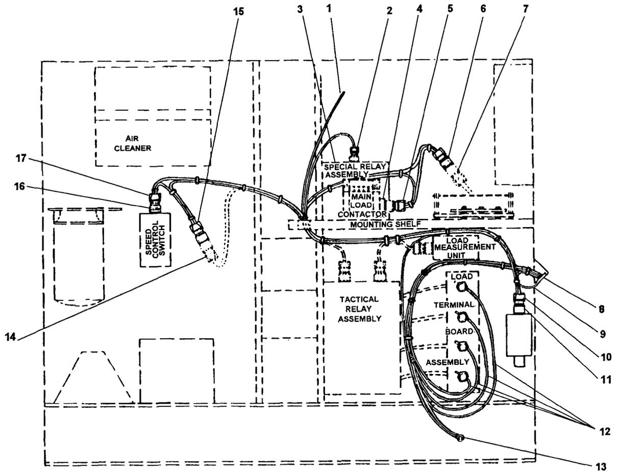
Figure 5-16. Applications Kit Cable Harness Assembly Installation (Right Side)
