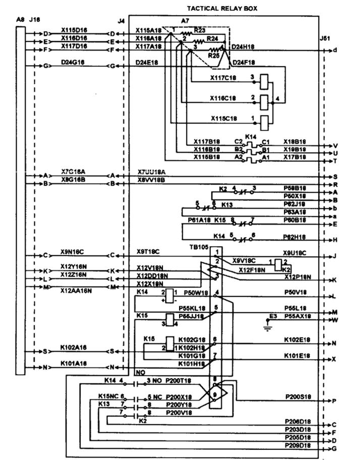
FO-1. AC and DC, 15 and 30 KW, 50/60 and 400 Hz, Precise and Utility, Wiring Diagram, Drawing No. 72-2205
