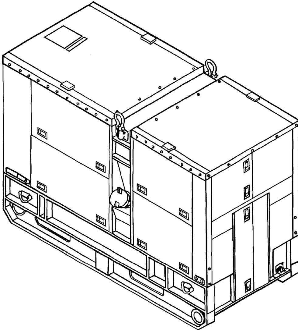
Figure 1-2. Engine Generator Set, Left-Rear, Three-Quarter View
