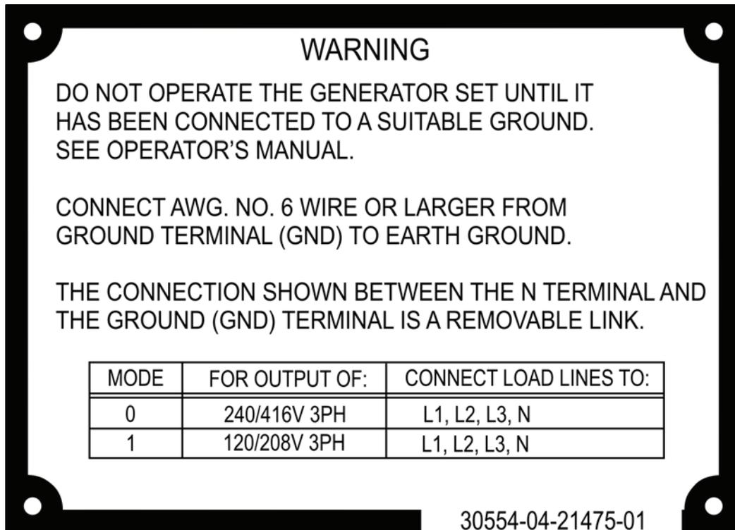
Figure 51. Label, Grounding Stud — Model 1060/1061.
