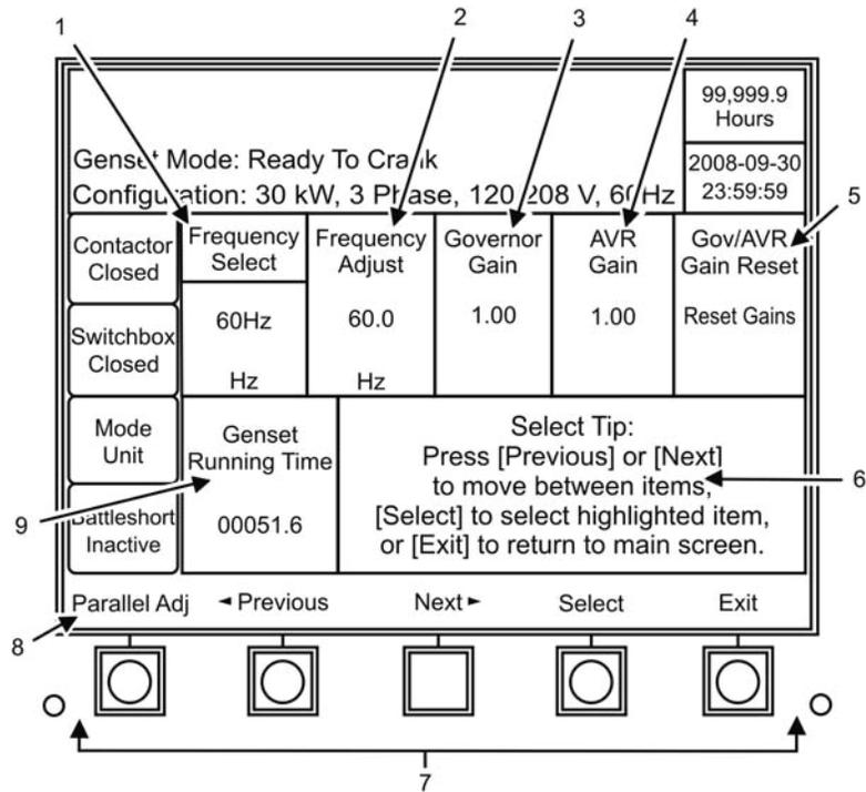
**Figure 11. [Adjustments] Screen 2 — Select Parameter.**
