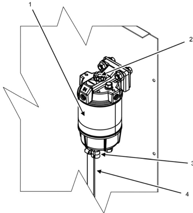
**Figure 3. Fuel Filter/Water Separator.**
