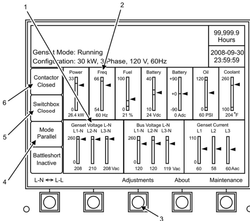
**Figure 4. Main Display Screen — Parallel Mode.**
