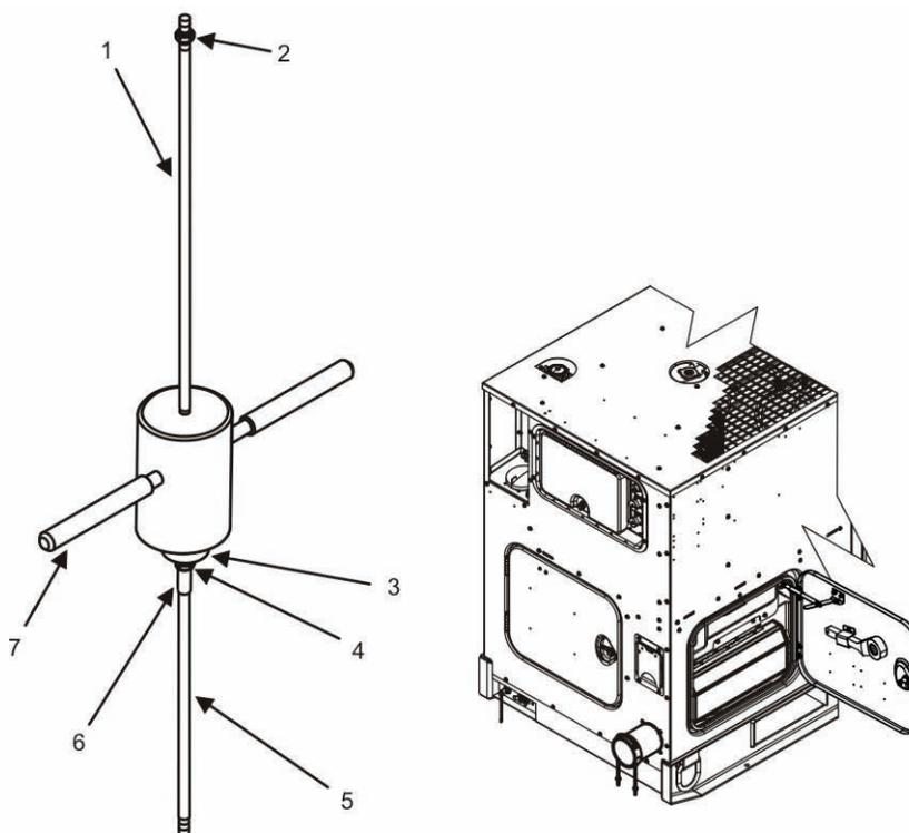
**Figure 3. Install Ground Rod With Slide Hammer.**
