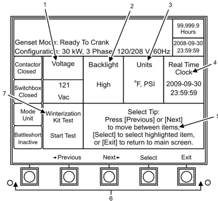
Figure 9. [Adjustments] Screen 1 — Select Parameter.
