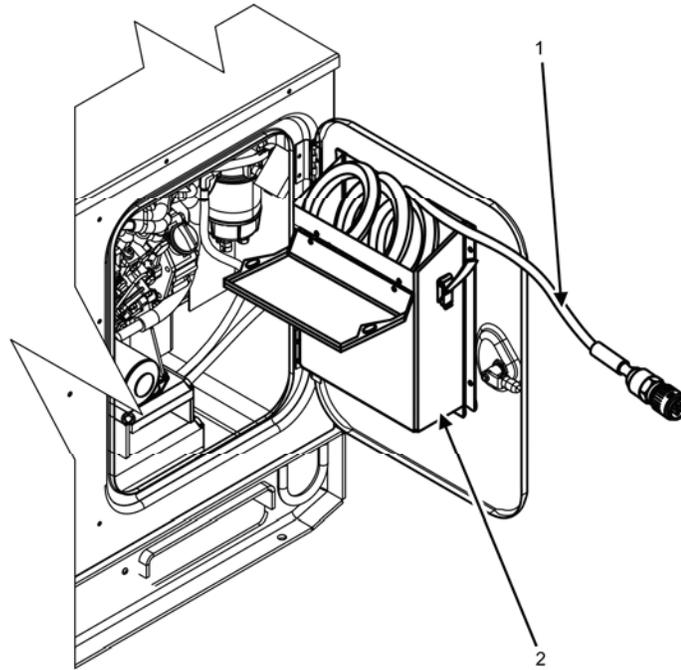
**Figure 1. Storage Box and Cable — Location.**
