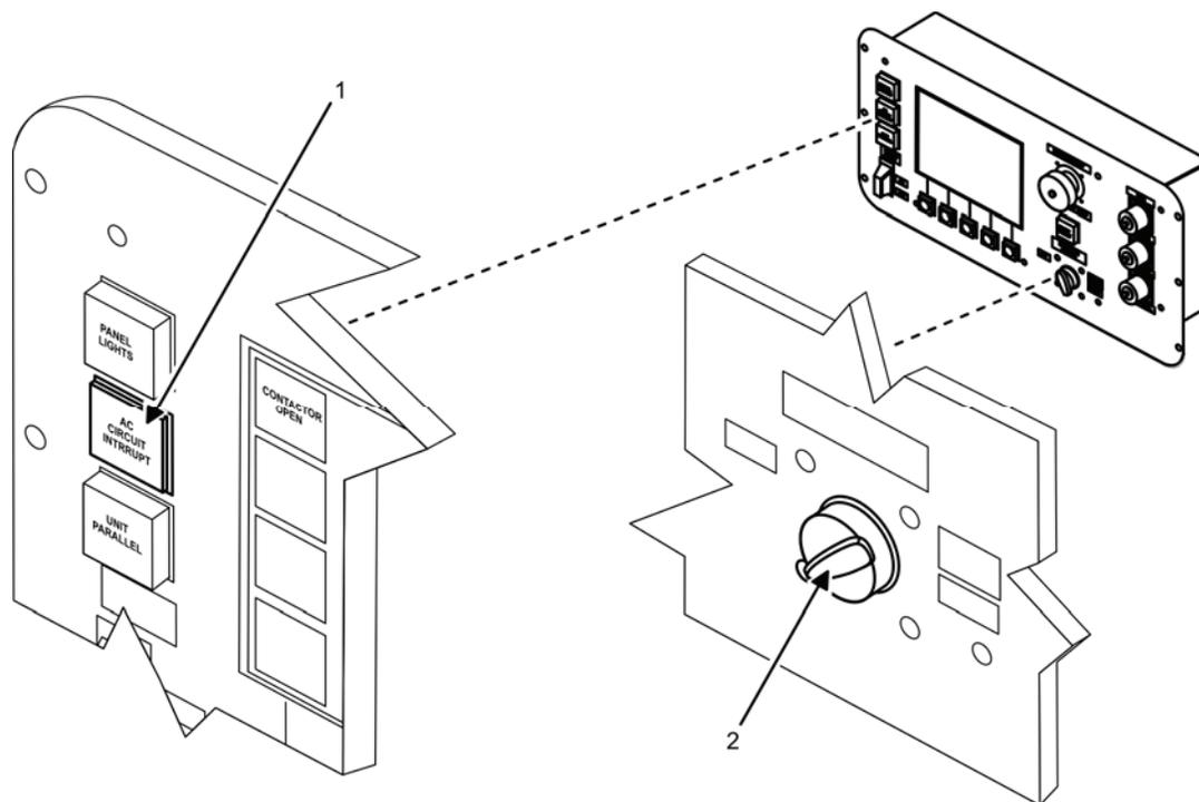
**Figure 27. Stopping Procedure.**
