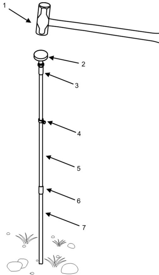
**Figure 4. Install Ground Rod With Sledge Hammer.**
