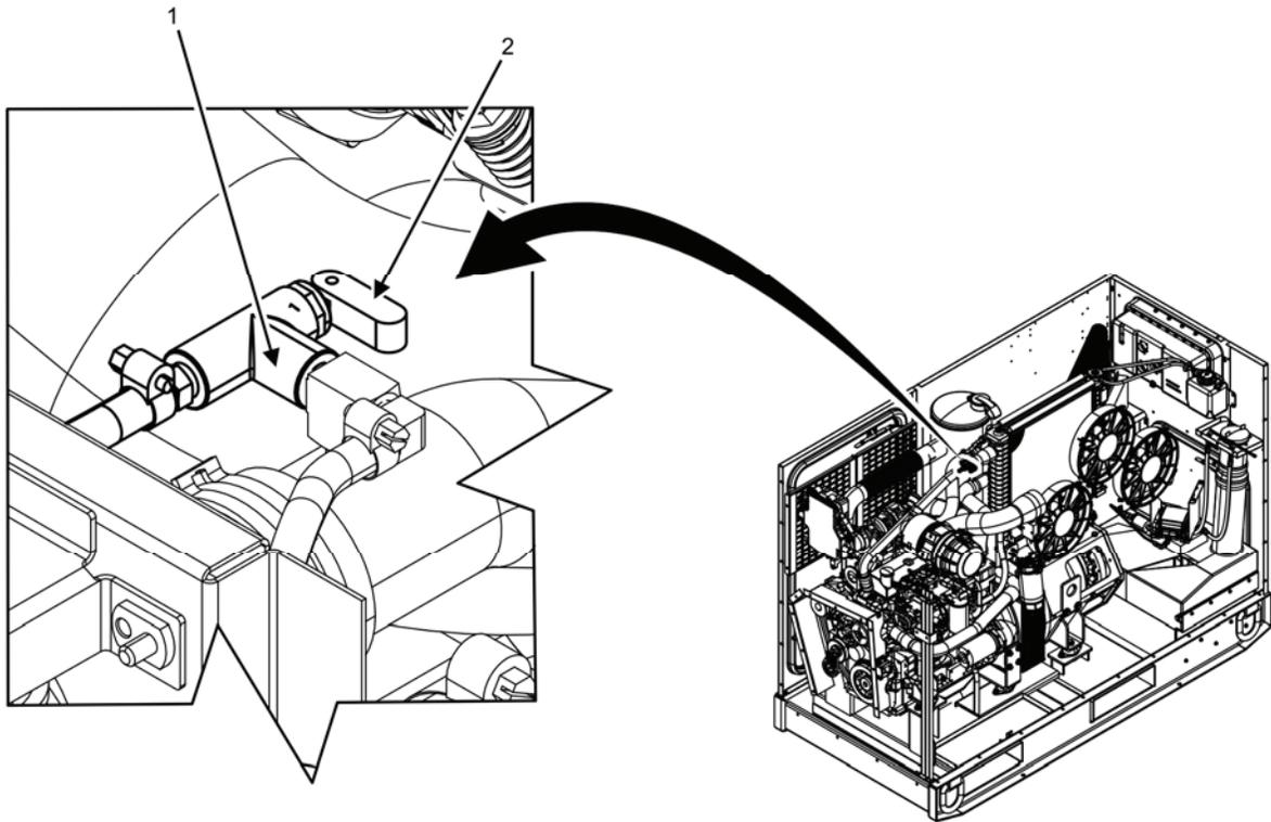
**Figure 6. Pressure Relief Valve.**
