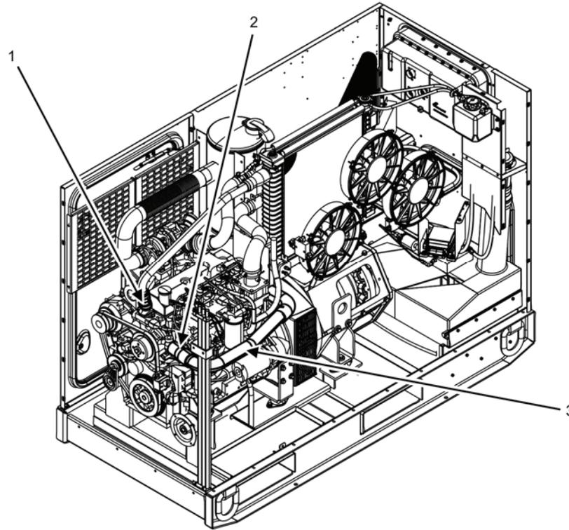
**Figure 7. Cooling System Hoses, Interconnecting Tubes, and Clamps — Left Side.**
