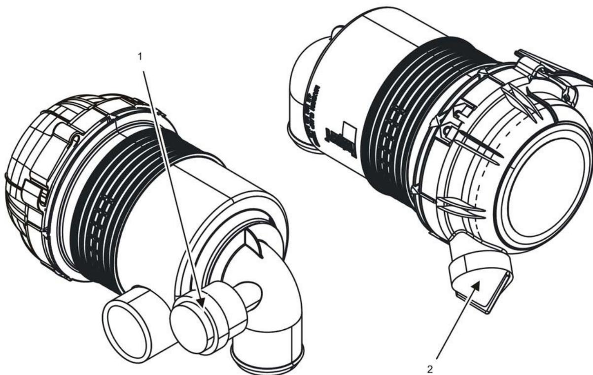
**Figure 2. Air Cleaner/Air Filter Restriction Indicator and Dust Ejector Valve.**
