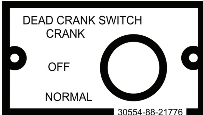
Figure 53. Label, Dead Crank — Model 1060/1061.
