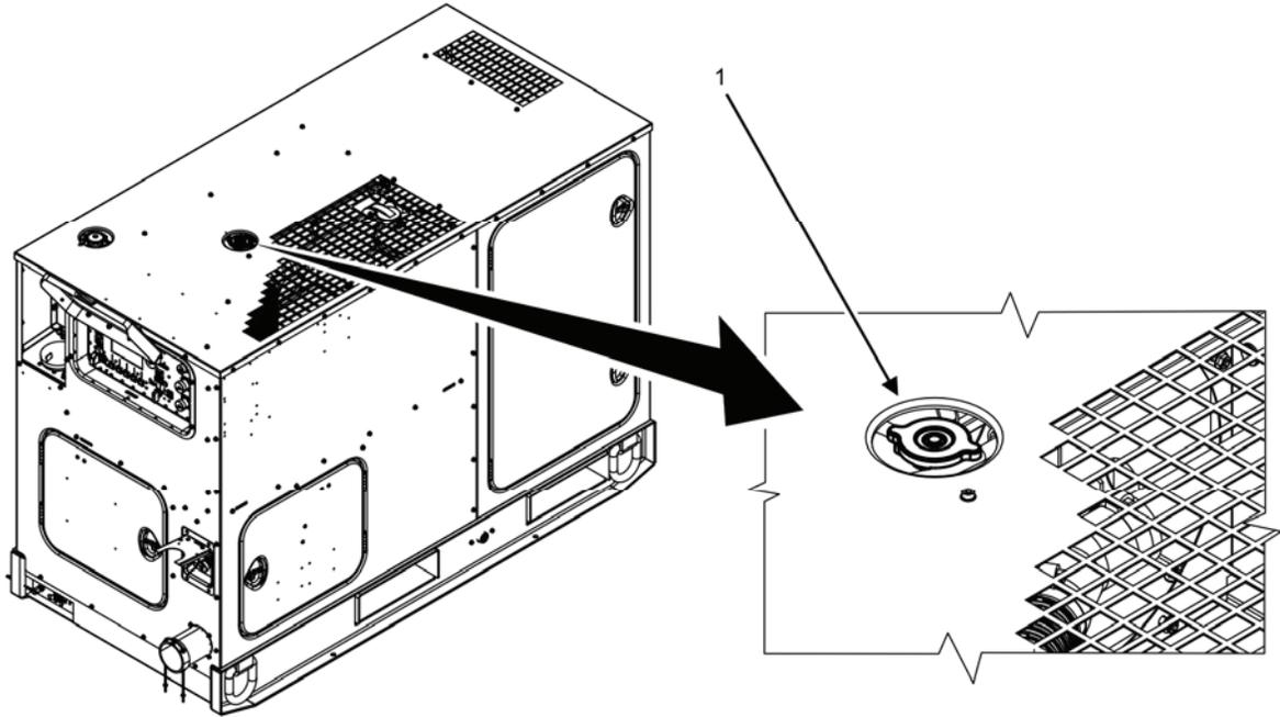
**Figure 4. Radiator Fill — Exterior.**
