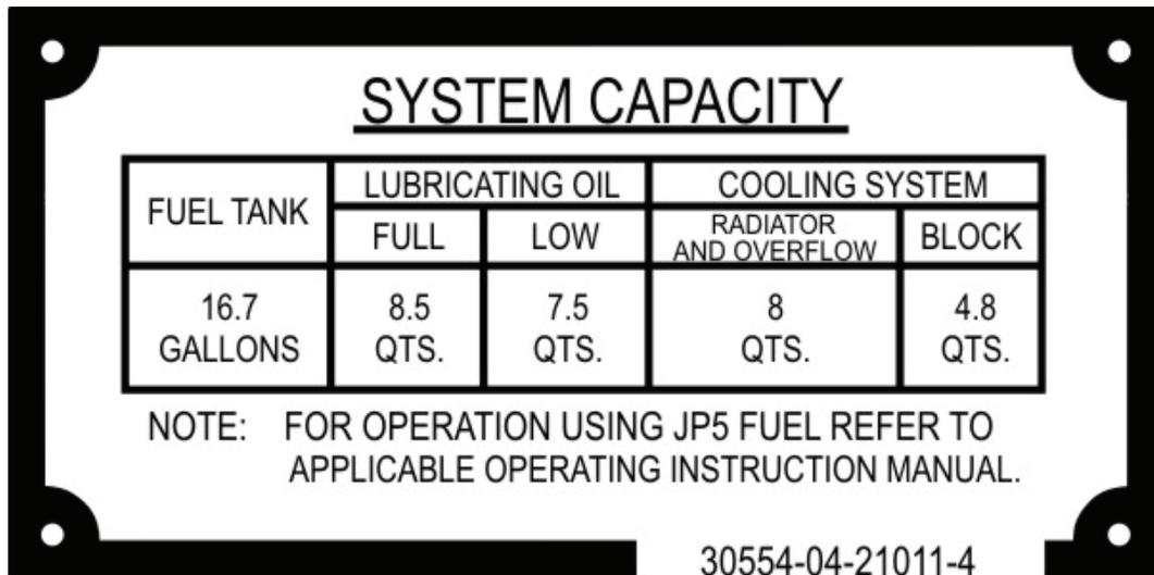
Figure 37. Plate, System Capacity — Model 1060/1061.
