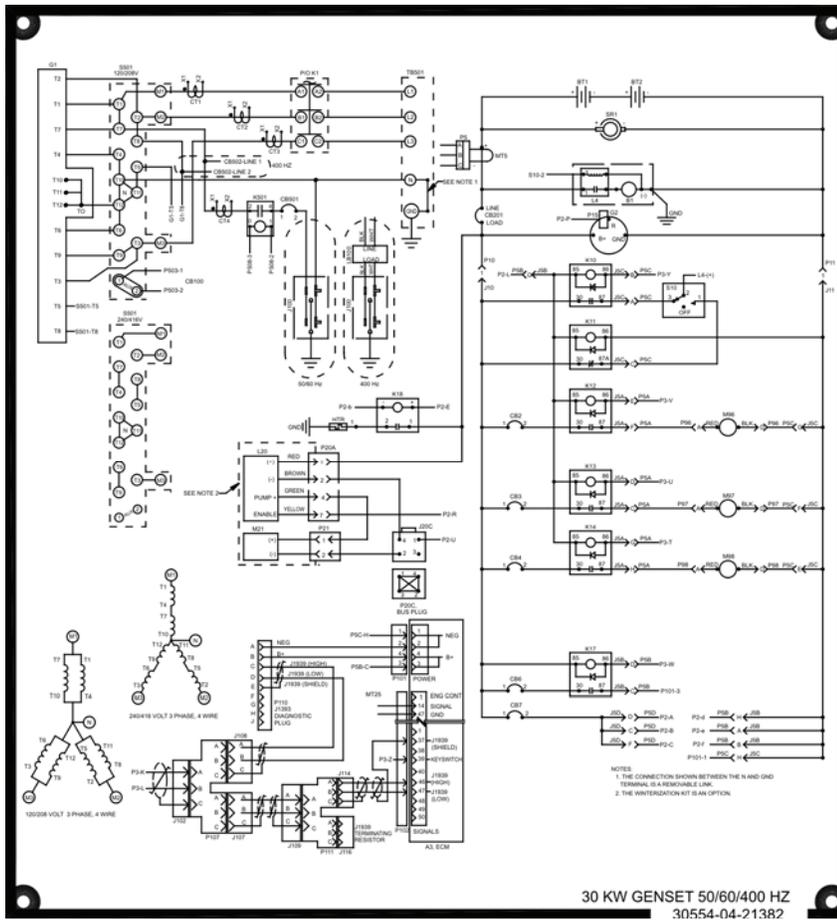
Figure 49. Label, Diagram, Wiring — Model 1060/1061.
