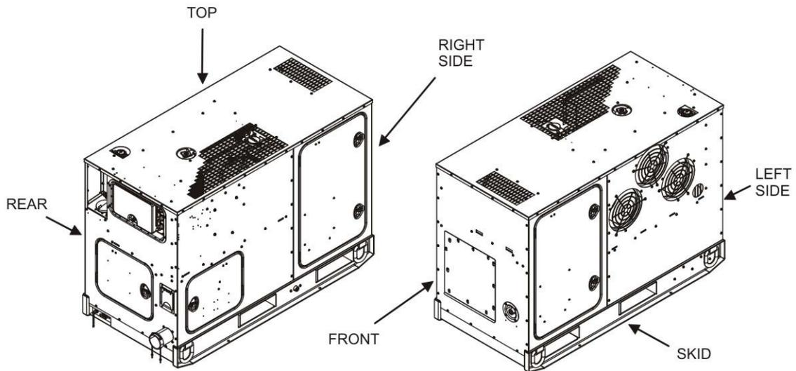
**Figure 1. Skid-Mounted 30 kW AMMPS Generator Set.**
