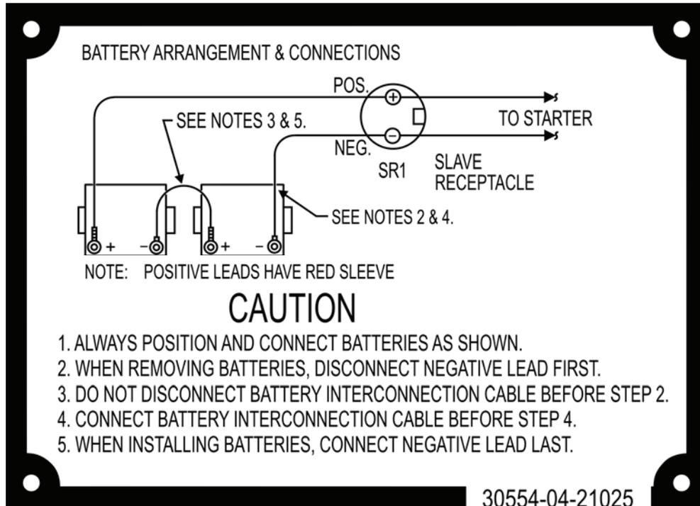
Figure 55. Label, Battery Connection — Model 1060/1061.
