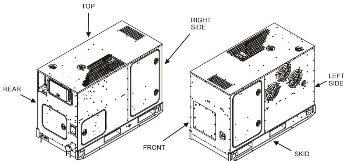
**Figure 1. AMMPS 30 kW Generator Set With Doors Closed.**
