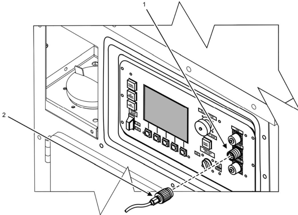
**Figure 24. Operator Display Panel — Remote Connection.**
