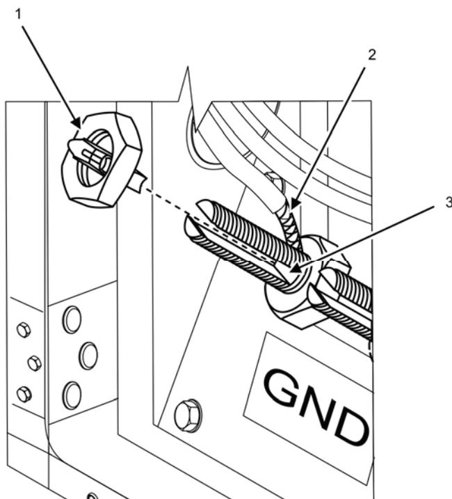
**Figure 7. Ground and Output Cable Attachment Detail.**
