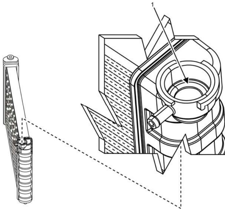
**Figure 5. Radiator Fill — Interior.**
