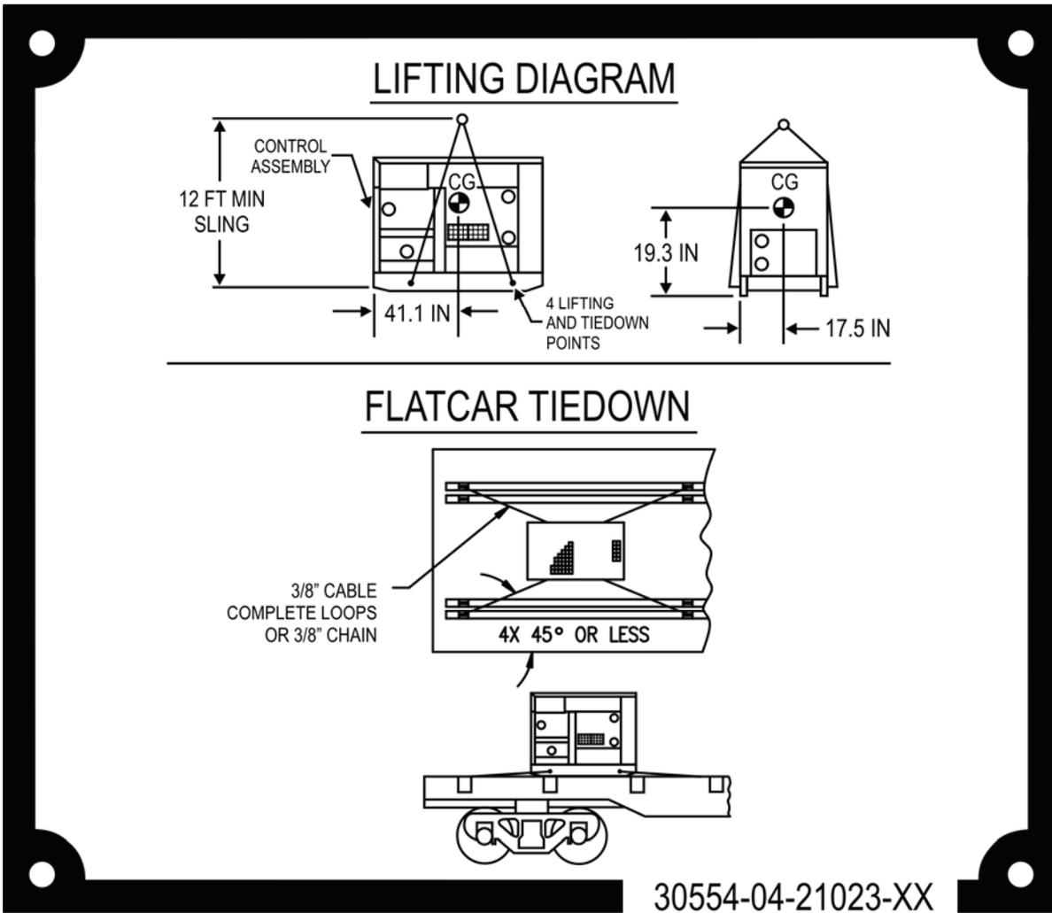
Figure 38. Label, Lifting and Tie Down — Model 1060/1061.
