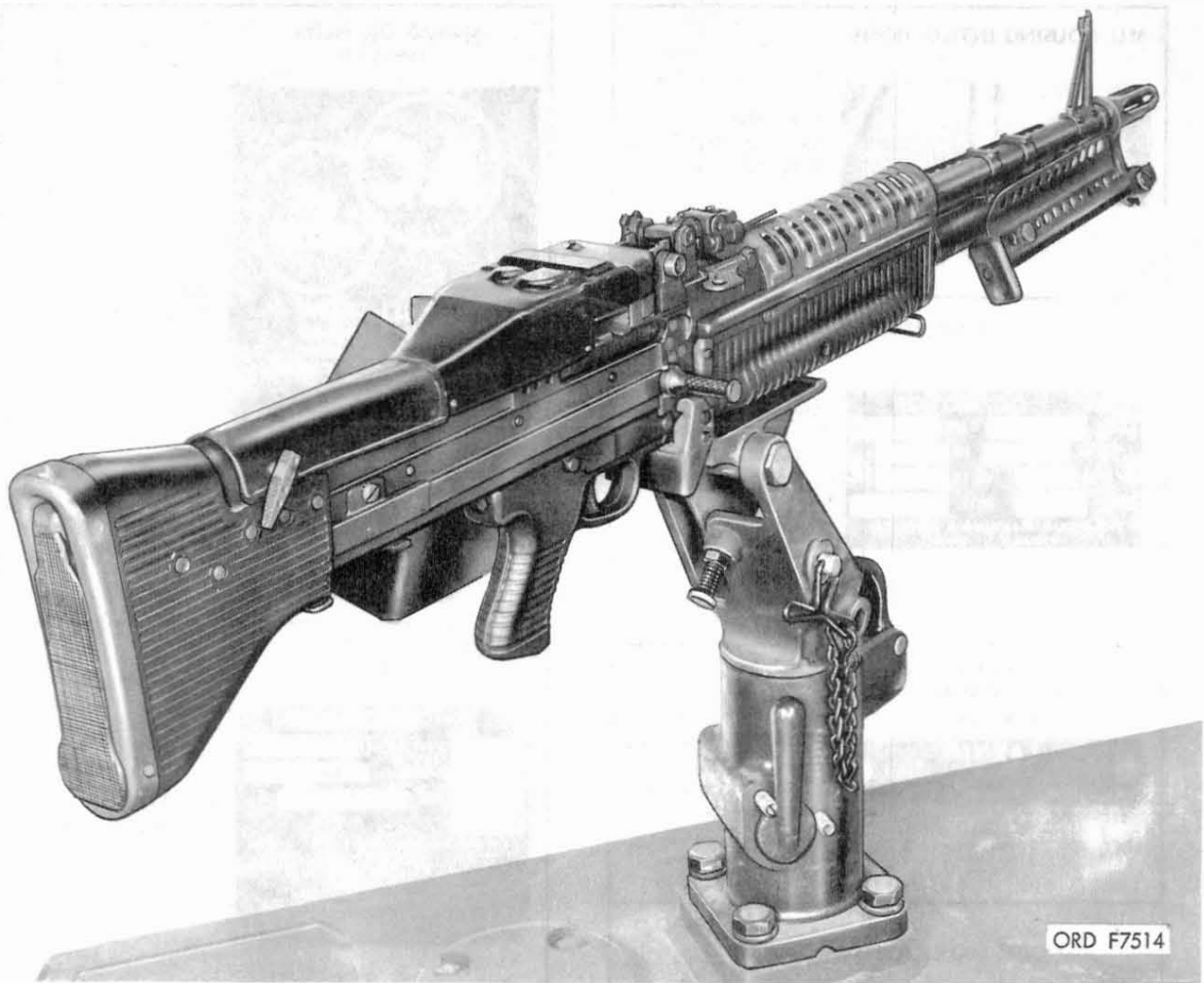
Figure 12. 7.62-mm machine gun M60 mounted on gun mount M142
