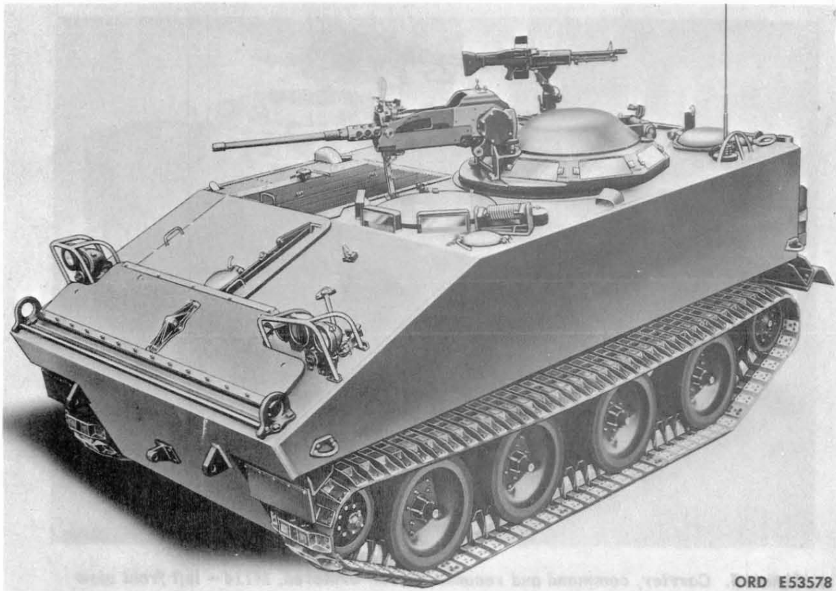
Figure 8. Carrier, command and reconnaissance: armored, M114A1 vehicle - left front view
