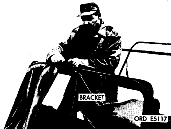
Figure 2-23. Canvas top sliding through slot.
