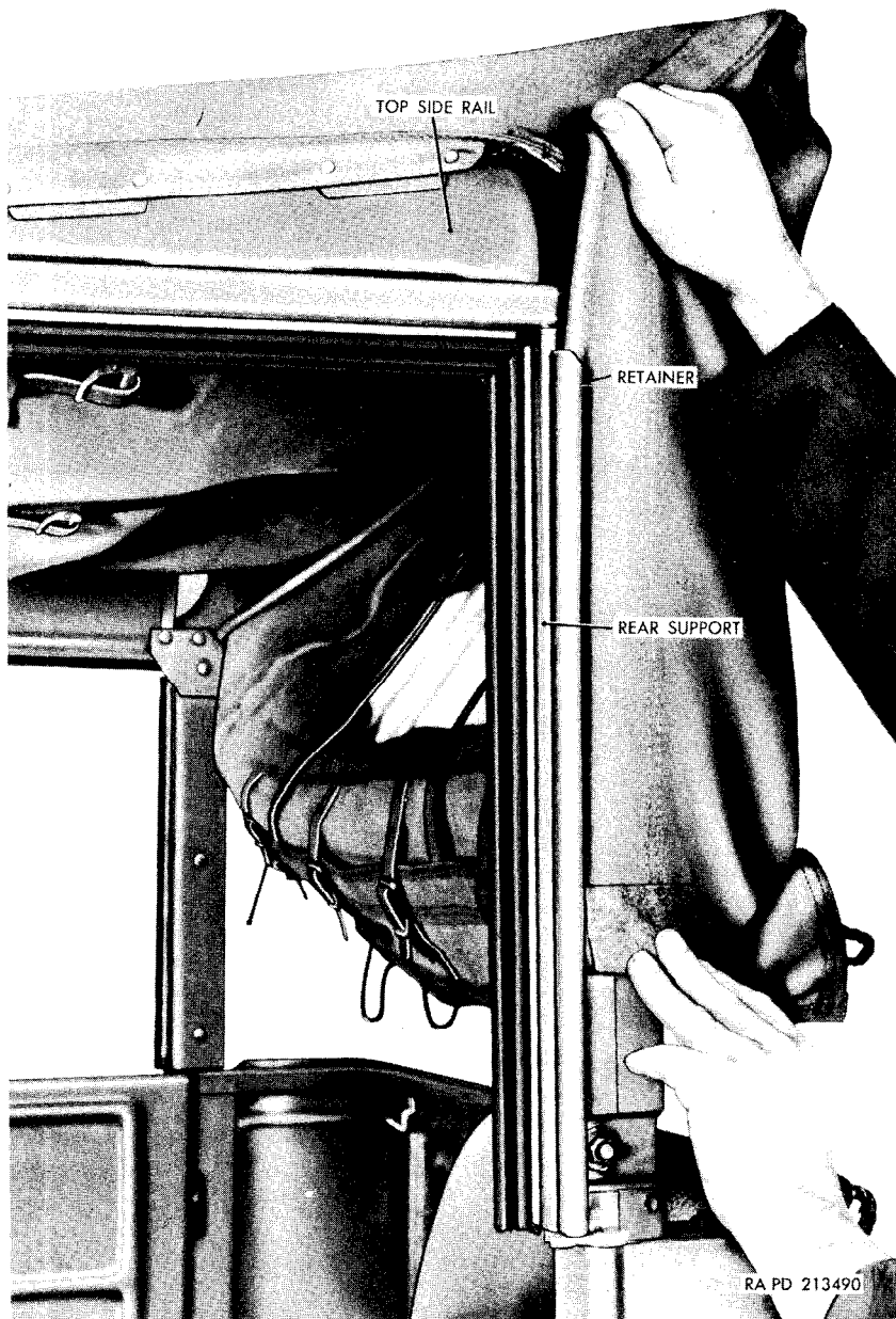
Figure 222. Removing top cover from side rail support.
