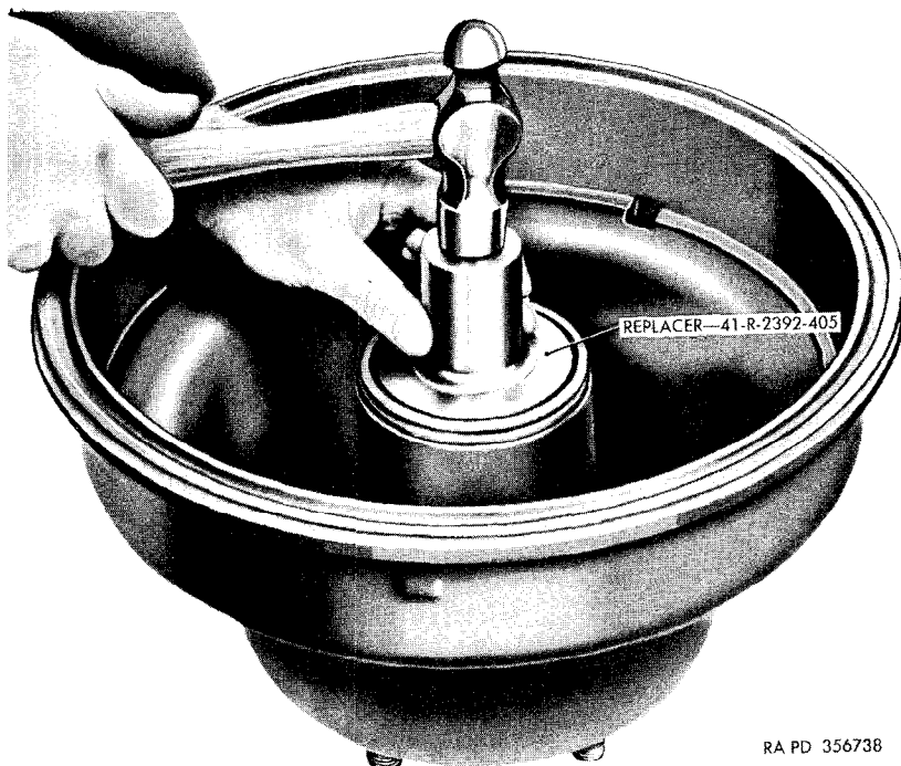
Figure 193. Installing inner bearing oil seal.
