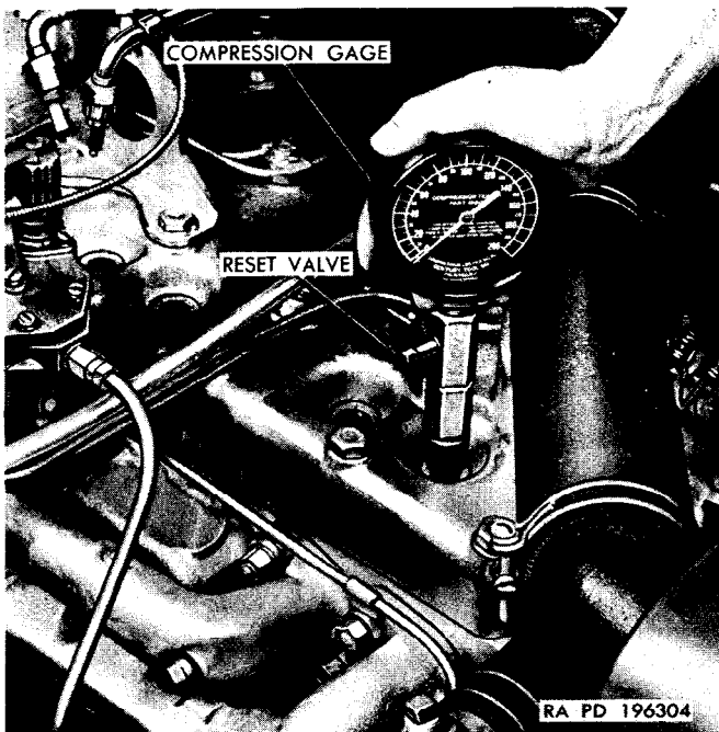
Figure 71. Engine compression test.
