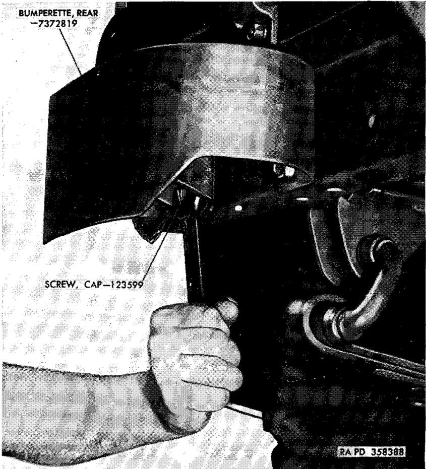
*Figure 20. Removing rear bumperettes and lifting shackles.*
