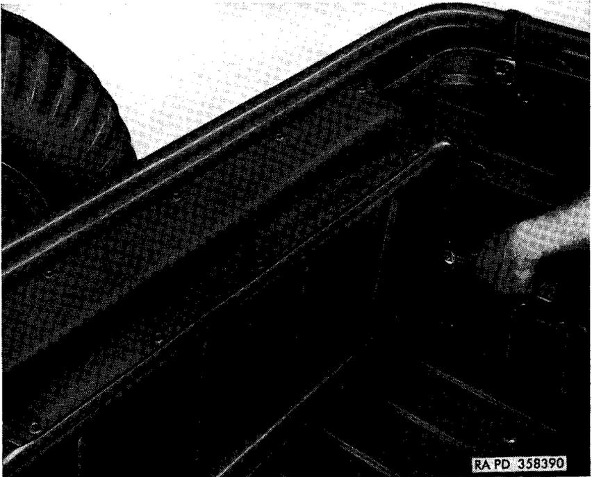
*Figure 16. Removing nut securing rear seat pivot tube retainer.*
