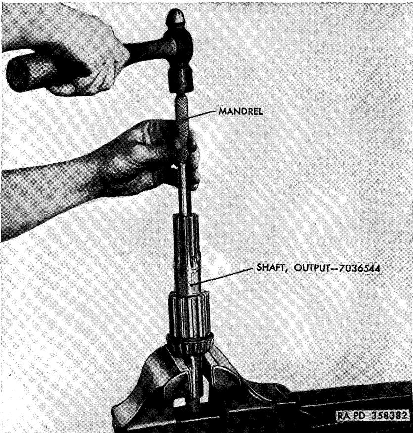
Figure 39. Replacing output clutch gear shaft pilot bearing.
