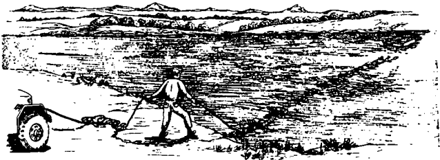
Figure 114. Floating winch cable to object of recovery.
