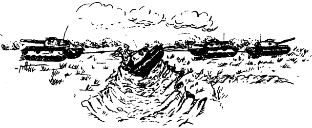
Figure 51. Recovering nosed tank with similar vehicles.
