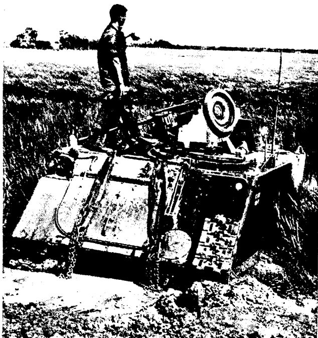
Figure 74. Two sling legs attached to each front towing lug.
